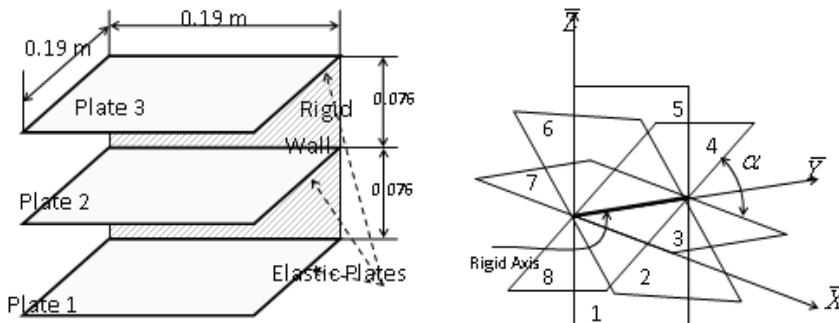
Figure 10: (a) A set of parallel plates fixed at one side, (b) A set of radial plates
