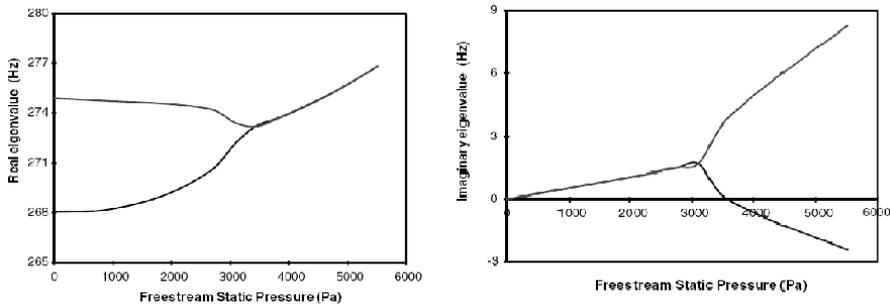
Figure 18: Eigenvalues of system vs freestream static pressure
