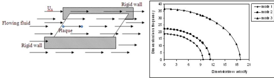
Figure 11: (a) Plate clamped on two opposite edges subjected to flowing fluid, (b) Variation of frequency versus fluid velocity
