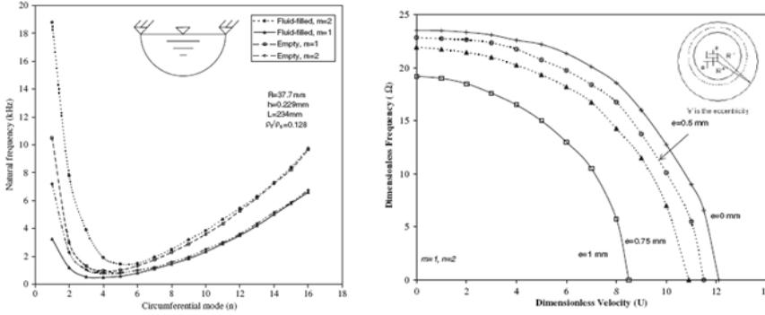
Figure 6: (a) Natural frequencies of an empty and fluid-filled open cylindrical shell as a function of circumferential mode number (b) Stability of a distorted cylindrical shell as a function of flow velocity
