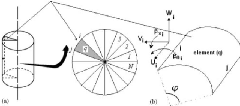
Figure 3: (a) Finite element discretization (N is the number of elements), (b) Nodal displacement at node ‘i’ of a typical element
