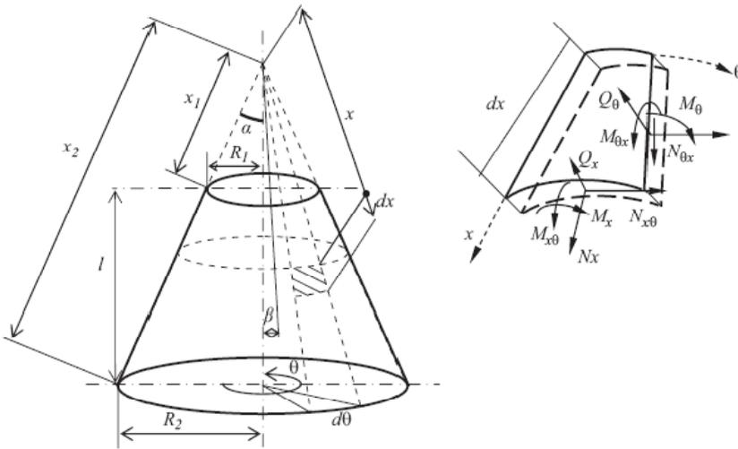
Figure 16: Geometry of a truncated conical shell
