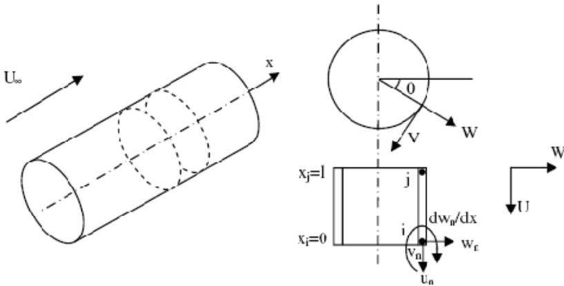
Figure 1: Geometry of cylindrical frustum element
