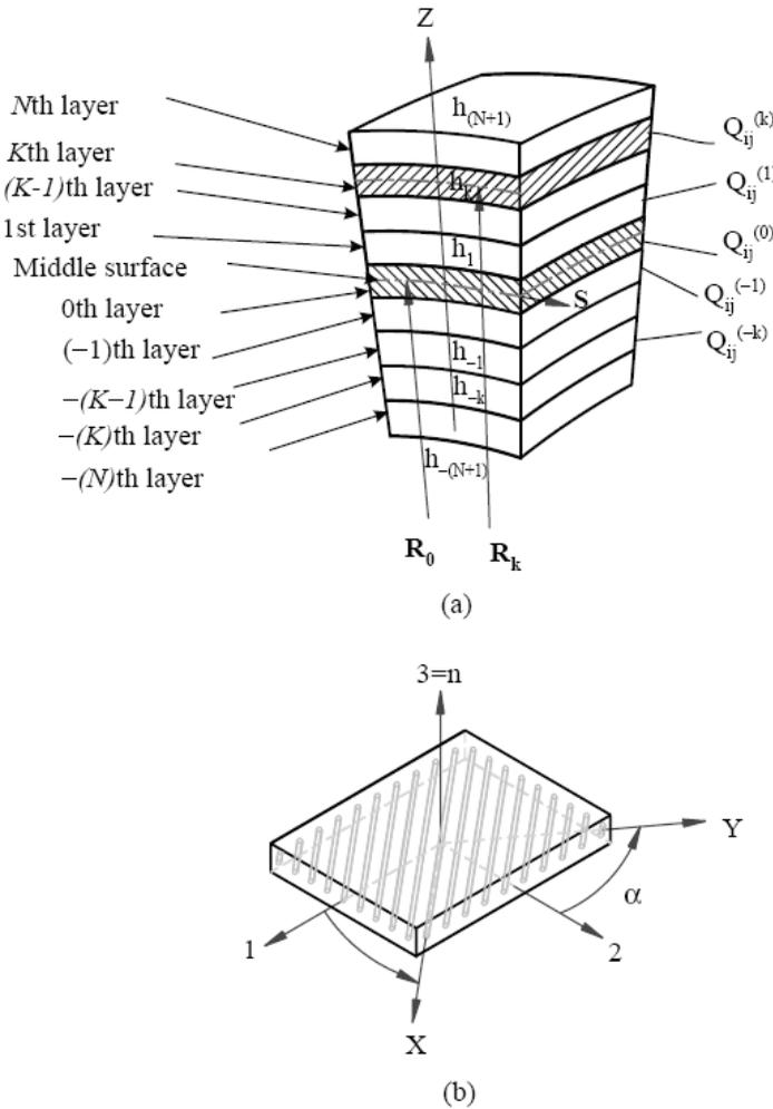
Figure 2: (a) Multi-directional laminate with co-ordinate notation of individual plies, (b) a fiber reinforced lamina with global and material co-ordinate system
