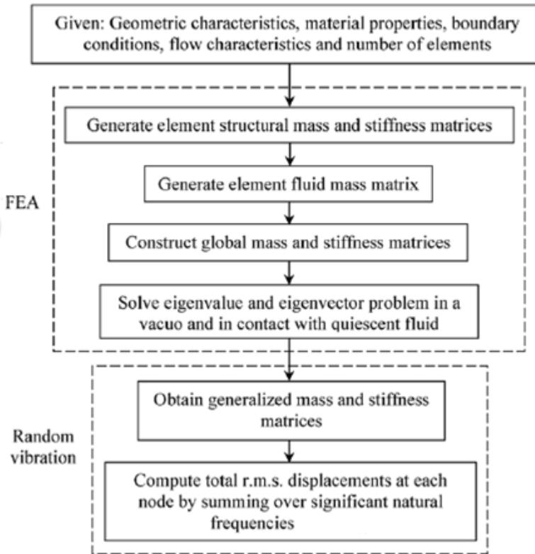
Figure 14: Flow chart of the computational process for calculation of root-mean square displacement response
