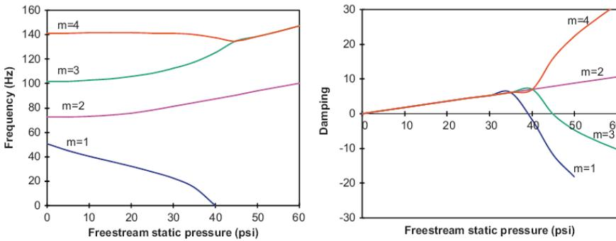
Figure 17: (a) Real part and (b) imaginary part of the complex frequencies versus freestream static pressure
