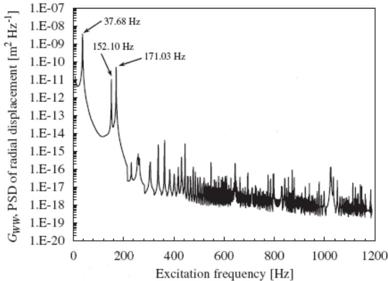
Figure 15: PSD of radial displacement of an SFSF plate subjected to fully developed turbulent flow
