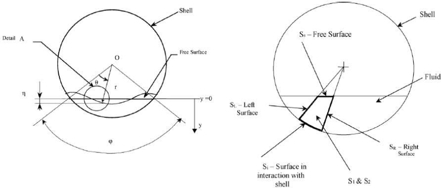
Figure 7: Slushing model of a horizontal shell (a) Modeling of free surface, (b) Free surfaces of a fluid finite element
