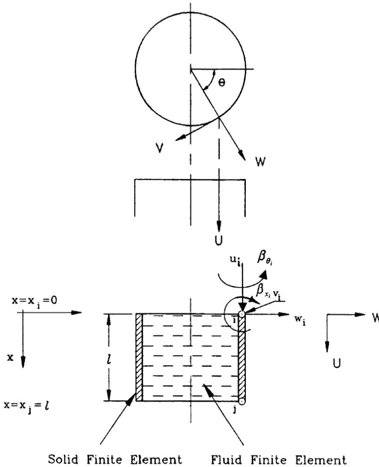
Figure 5: Displacement and degrees of freedom at a circular node
