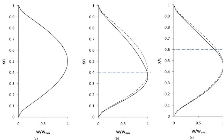
Figure 19: Variation of radial model shape ( $n=5$ ,  $m=1$ ) with filling ratio of a clamped-clamped shell under internal pressure  $P_m=1000$  Pa; a)  $H/L=0$ ; b)  $H/L=0.4$ ; c)  $H/L=0.6$ ; solid line: pressurized shell; dashed line: unpressurized shell
