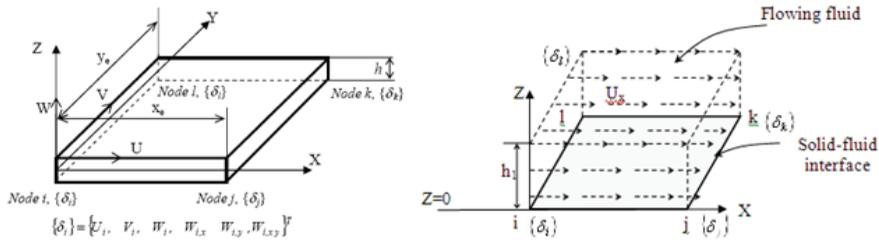
Figure 9: (a) Geometry and displacement field of a typical element, (b) Fluid-solid element
