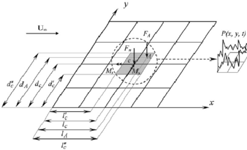
Figure 13: Transformation of a continuous pressure field into a discrete force field and the equivalent discrete force field acting at node c. Pressure fluctuations are also illustrated laterally on the area surrounding node c.
