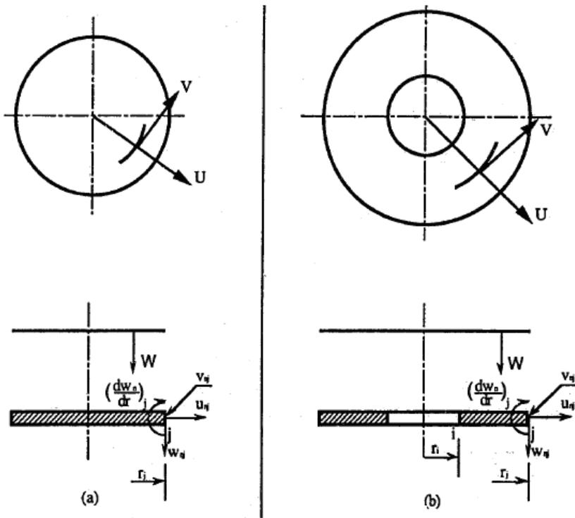
Figure 12: Displacement and degrees of freedom (a) Finite element of the circular plate type (b) Finite element of the annular plate type
