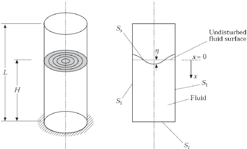
Figure 8: Slushing model of a vertical shell
