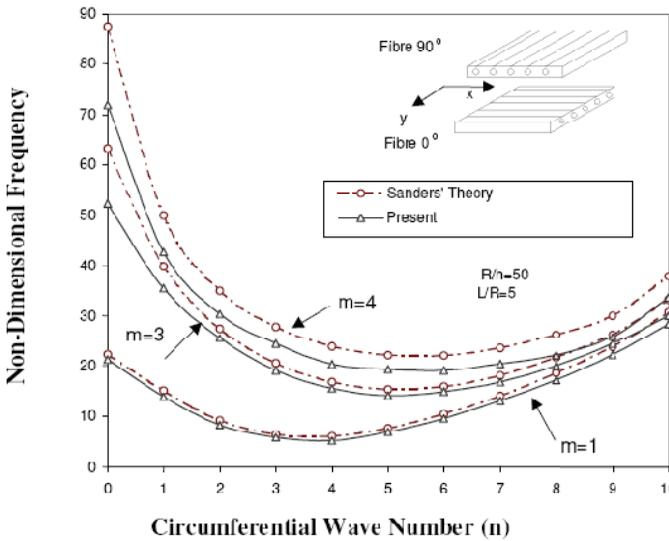
Figure 4: Variation of non-dimensional natural frequencies in conjunction with variation of m
