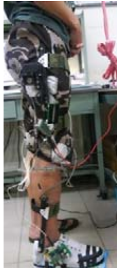
Figure 1: Lower-limb orthosis with curved spring
