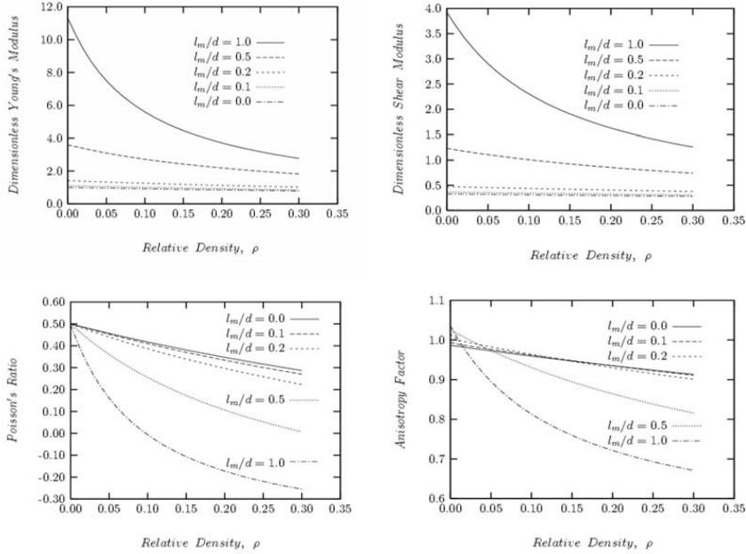
Figure 1: Elastic properties vs. the relative density of micro- open-celled foams: a) dimensionless Young's modulus  $\bar{E}_{11}$ ; b) dimensionless shear modulus  $\bar{G}_{12}$ ; c) the Poisson ratio  $\nu_{12}$ ; and d) the Zener's anisotropy factor  $A^*$
