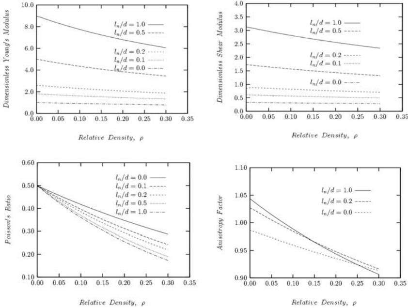
Figure 2: Effects of surface elasticity on the relationships between elastic properties and the relative density of nano-sized open-celled foams: a) dimensionless Young's modulus  $\bar{E}_{11}$ ; b) dimensionless shear modulus  $\bar{G}_{12}$ ; c) the Poisson ratio  $\nu_{12}$ ; and d) the Zener's anisotropy factor  $A^*$ .
