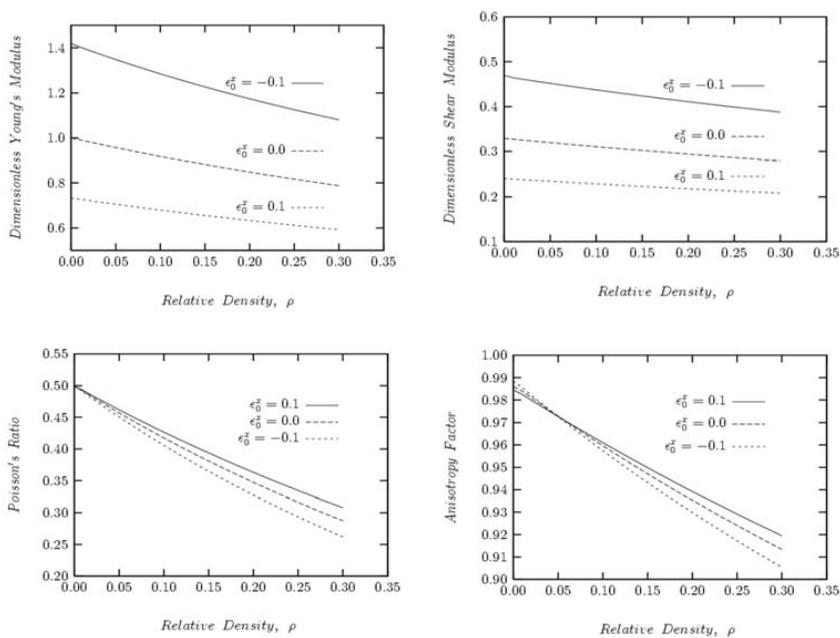
Figure 3: The elastic properties vs. the relative density of nano-sized open-celled foams: a) dimensionless Young's modulus  $\bar{E}_{11}$ ; b) dimensionless shear modulus  $\bar{G}_{12}$ ; c) the Poisson ratio  $\nu_{12}$ ; and d) the Zener's anisotropy factor  $A^*$ .
