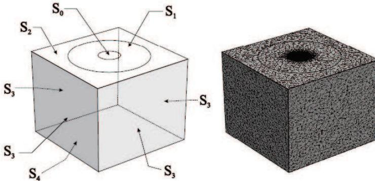
Figure 2: The sub-cube model of the porous medium with the annular permeameter. [Selvadurai and Selvadurai, 2010]
