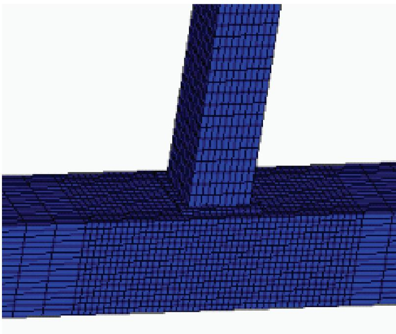
Figure 8: FE mesh of a collar-plate reinforced square tubular T-joint
