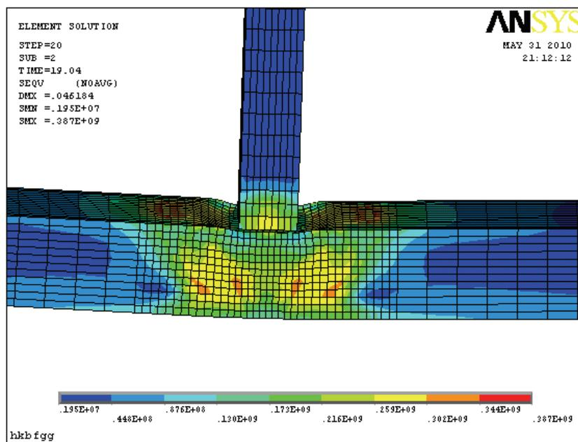
Figure 10: Stress distribution of the reinforced specimen
