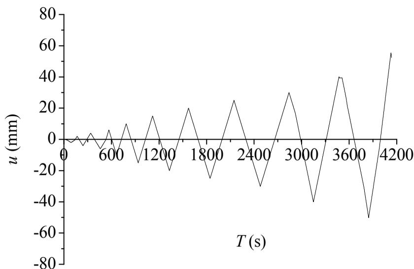
Figure 5: Loading scheme for collar-plate reinforced specimen
