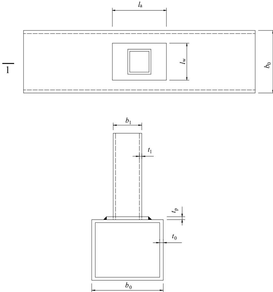
Figure 1: Configuration of a square tubular T-joint with collar plate reinforcement
