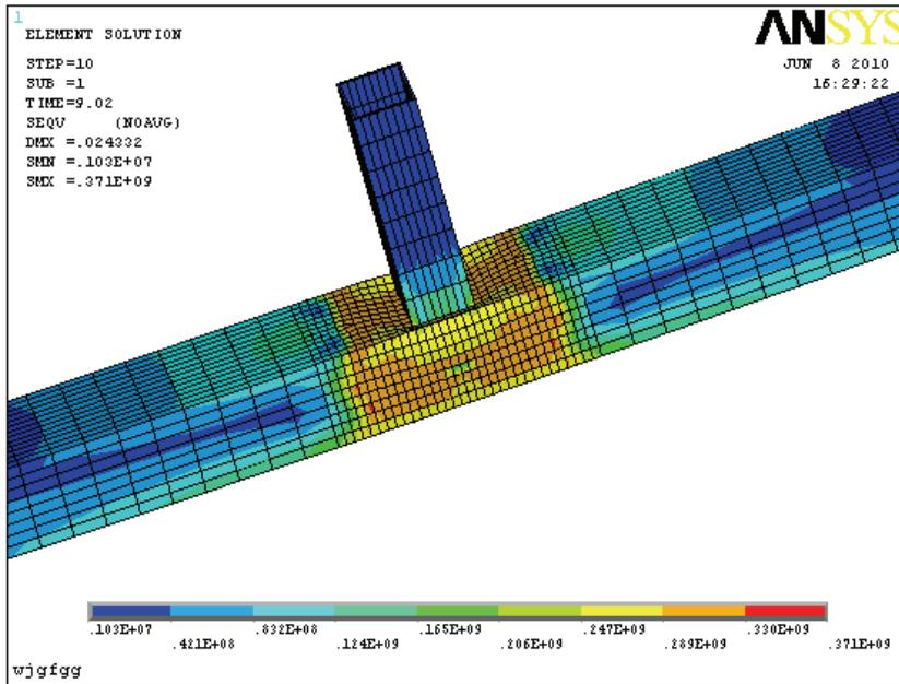
Figure 9: Stress distribution of the un-reinforced specimen
