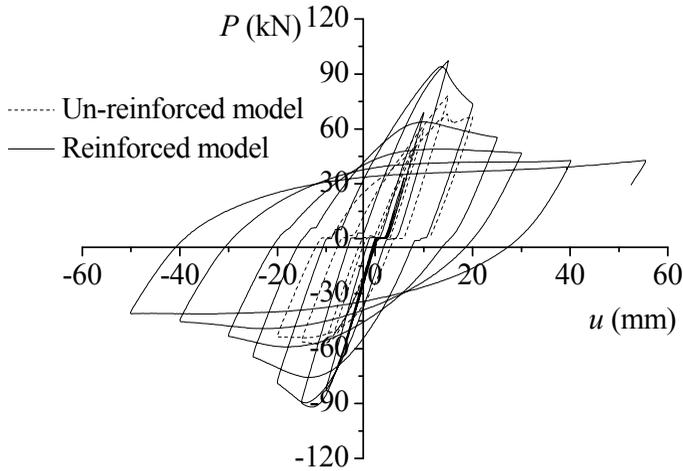
Figure 13: Comparison of the experimental hysteretic curves
