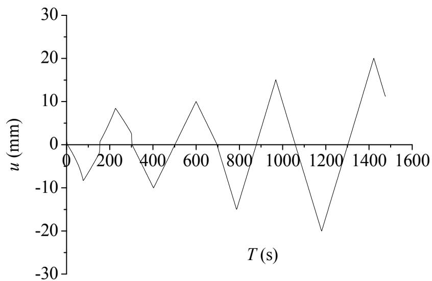
Figure 4: Loading scheme for un-reinforced specimen
