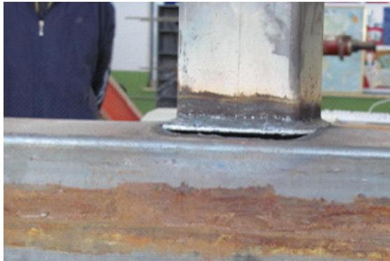
(b) final fracture failure
