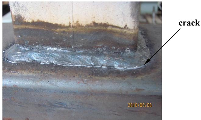
(a) initiation and propagation of crack along the weld toe
