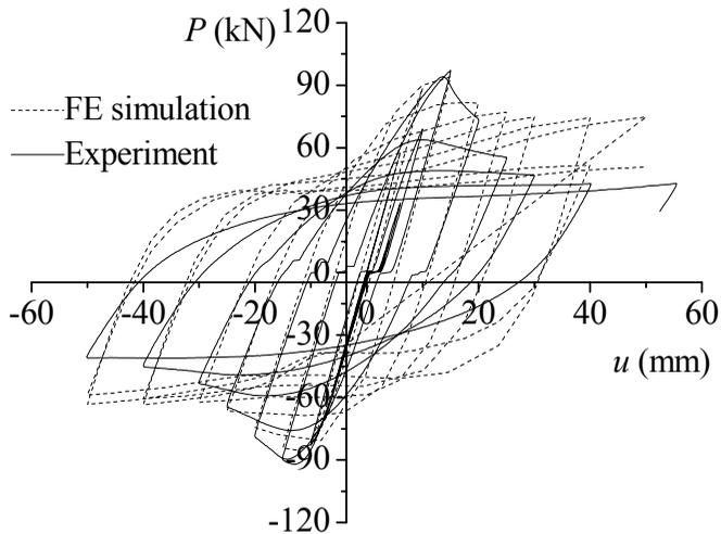
Figure 12: Hysteretic curves of the reinforced T-joint
