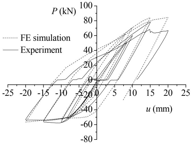
Figure 11: Hysteretic curves of the un-reinforced T-joint
