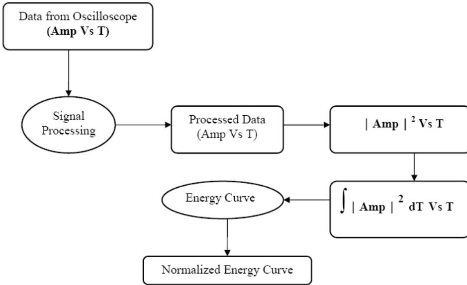
Figure 5: Block diagram for formation of Normalized Energy Curves
