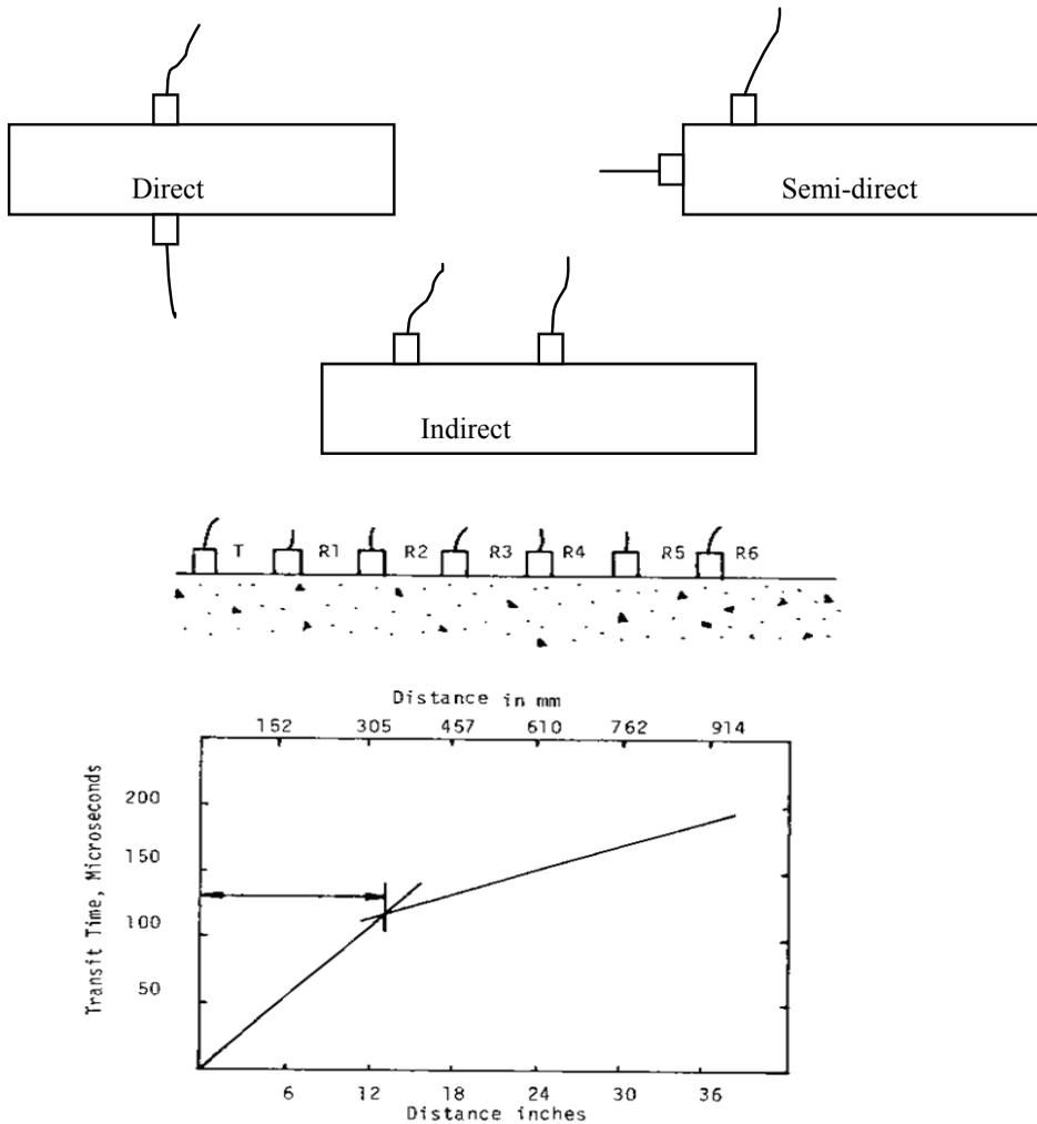
Figure 1: Use of one-sided pulse velocity (indirect) test to quantify depth of degradation [Malhotra, Carino (2004)]
