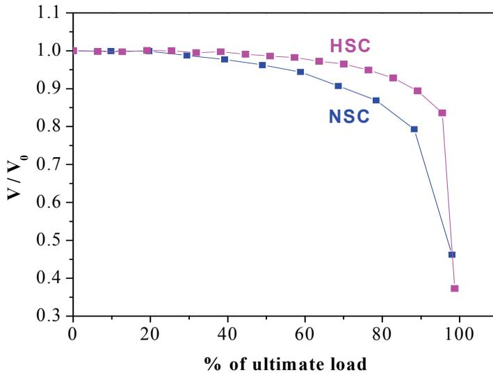
Figure 7: Variation of the pulse velocity with the load level
