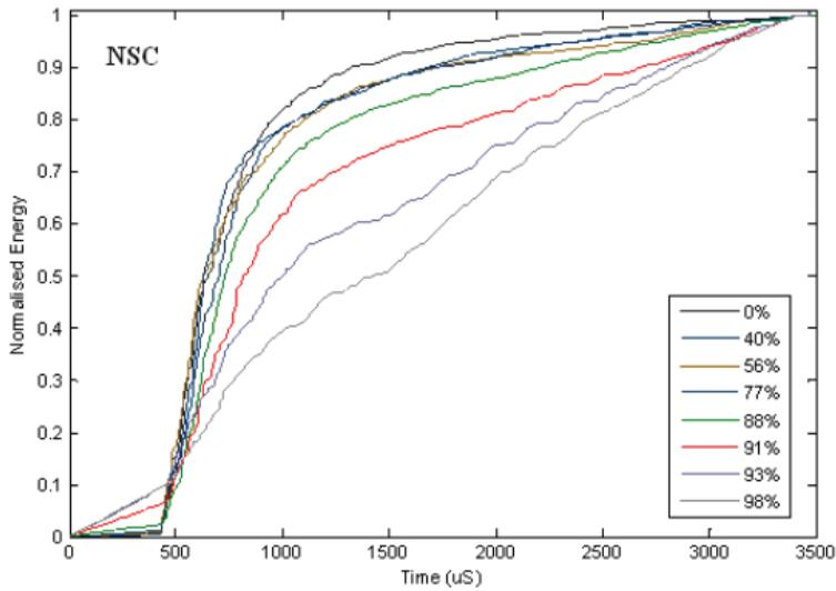
Figure 11: Normalized energy curves at different load levels for NSC
