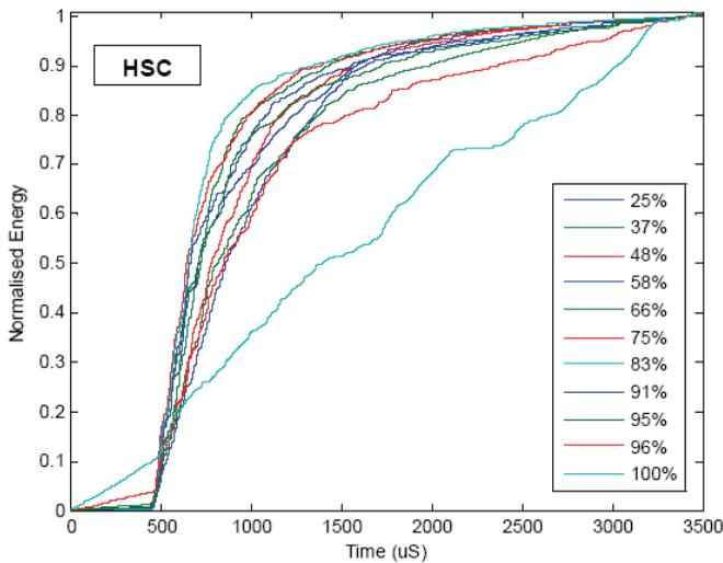
Figure 12: Normalized energy curves at different load levels for HSC
