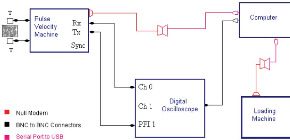
Figure 3: Experimental set up for obtaining A-scan
