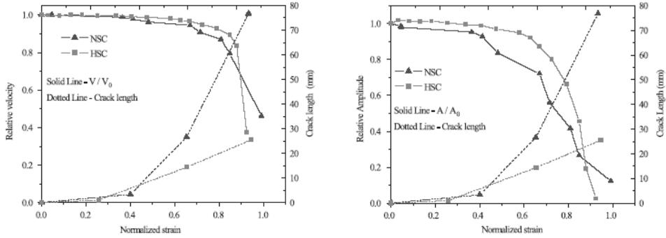
Figure 10: Variation of ultrasonic parameters (velocity and amplitude) and crack length [9] with strain levels in concrete under uniaxial compression
