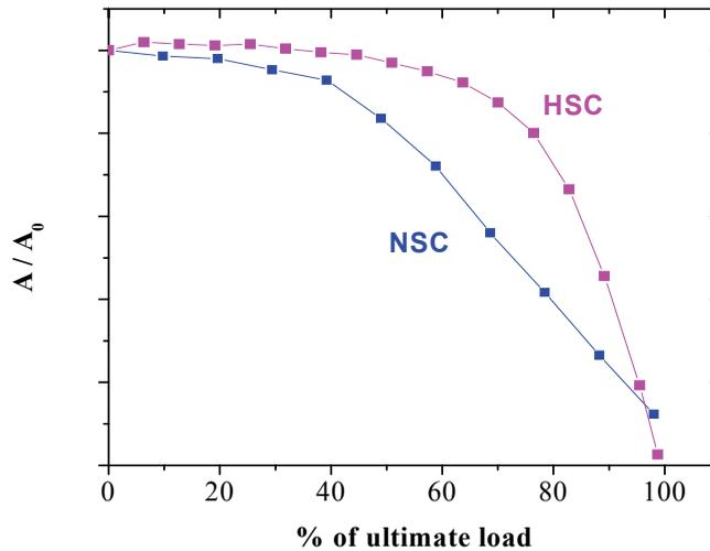
Figure 9: Variation of pulse amplitude with the load level
