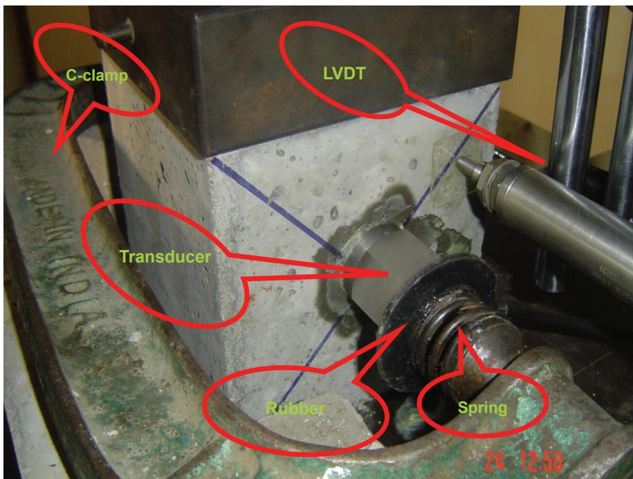
Figure 2: Experimental setup for ultrasonic measurements
