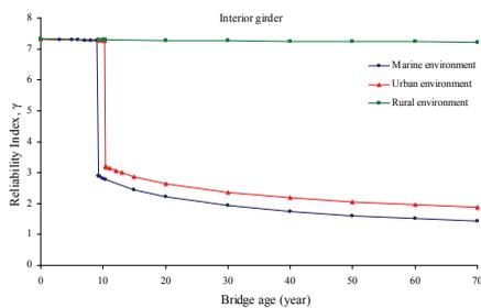
Figure 10: Variation in reliability index with age in different environments for interior girder.
