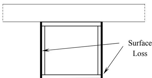
Figure 1: Model of corroded steel box girder cross-section.
