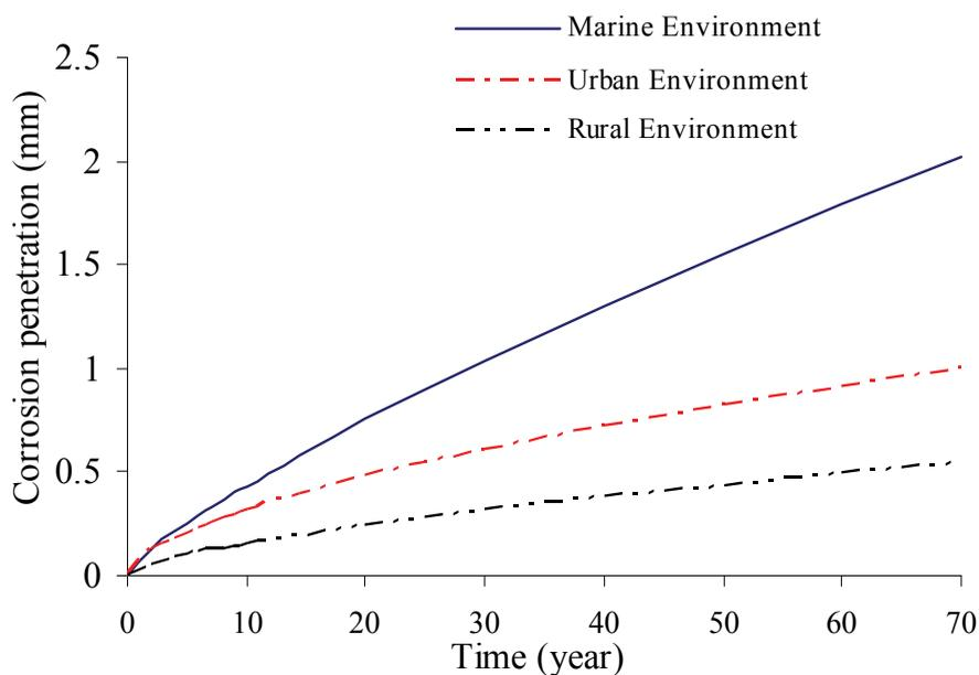
Figure 2: Corrosion penetration versus time for carbon steel in various environments.
