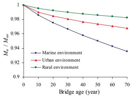
Figure 9: Variation of box ultimate strength with age in different environments.
