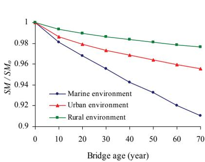
Figure 8: Variation of section modulus with age in different environments.
