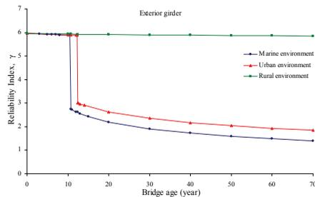
Figure 11: Variation in reliability index with age in different environments for exterior girder.
