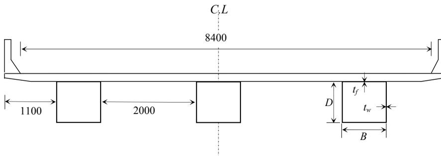
Figure 6: Typical cross-section of box girder bridge (dimensions in mm).
