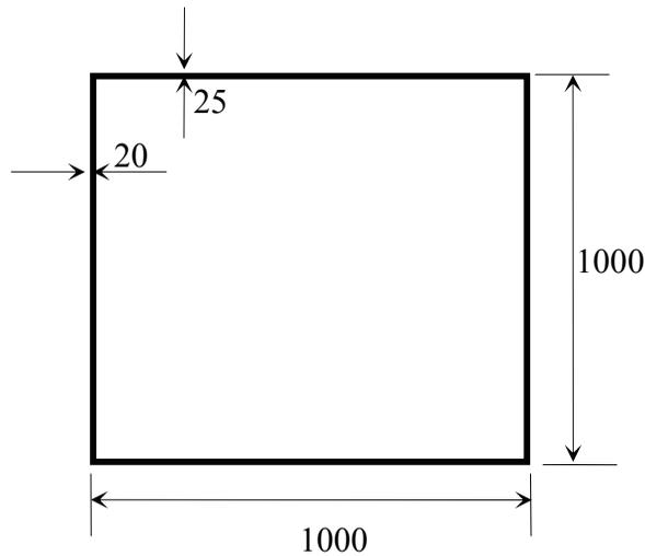
Figure 7: Dimensions (in mm) of cross-section of box girder.
