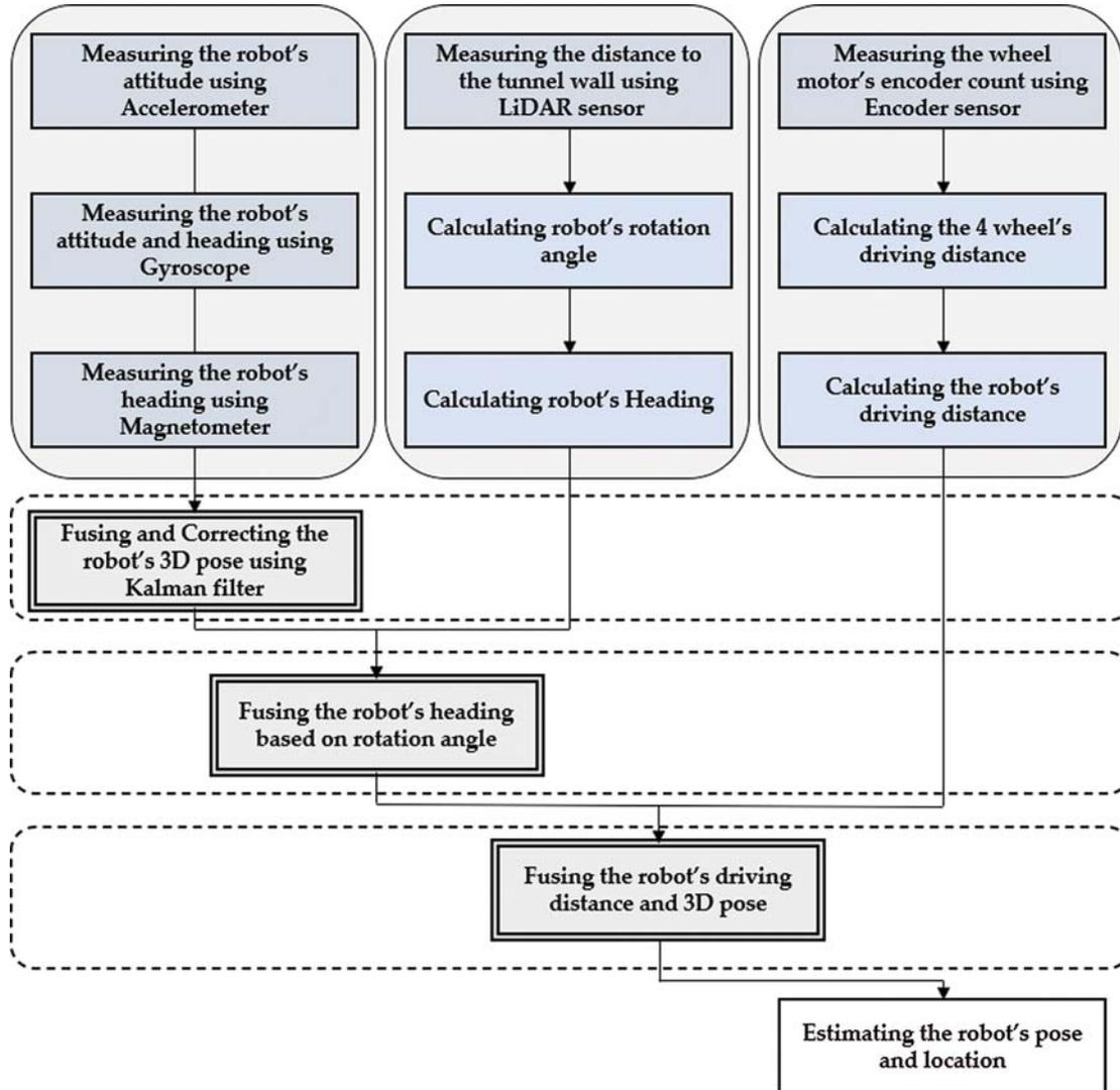
**Figure 8:** Overall system architecture of the data processing algorithm for location estimation
