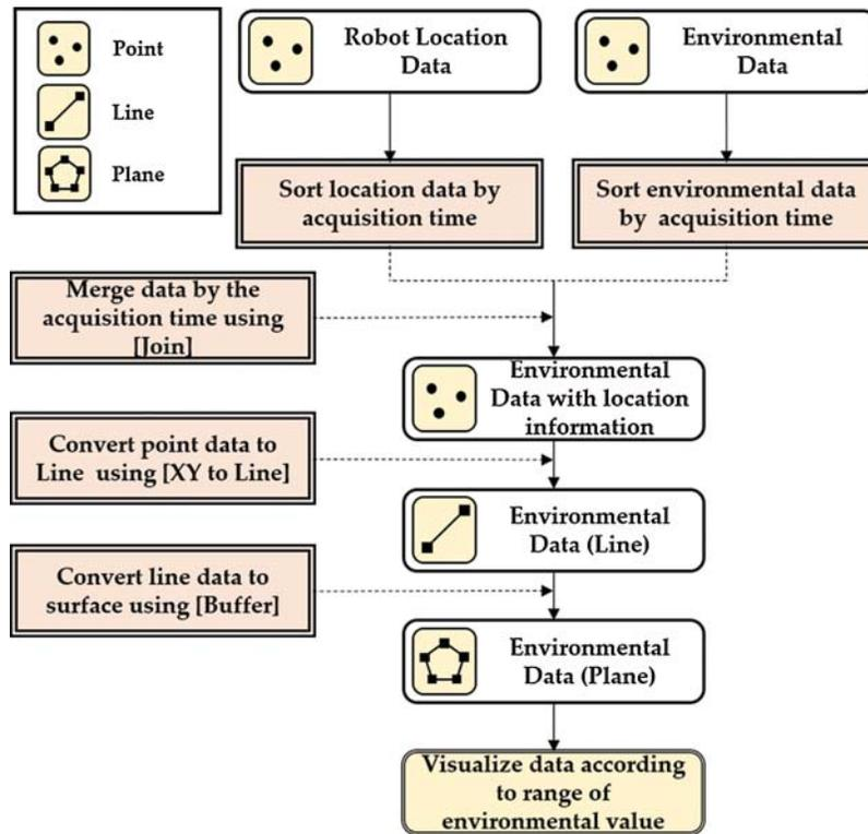
Figure 11: System architecture of environmental mapping system developed in this study
