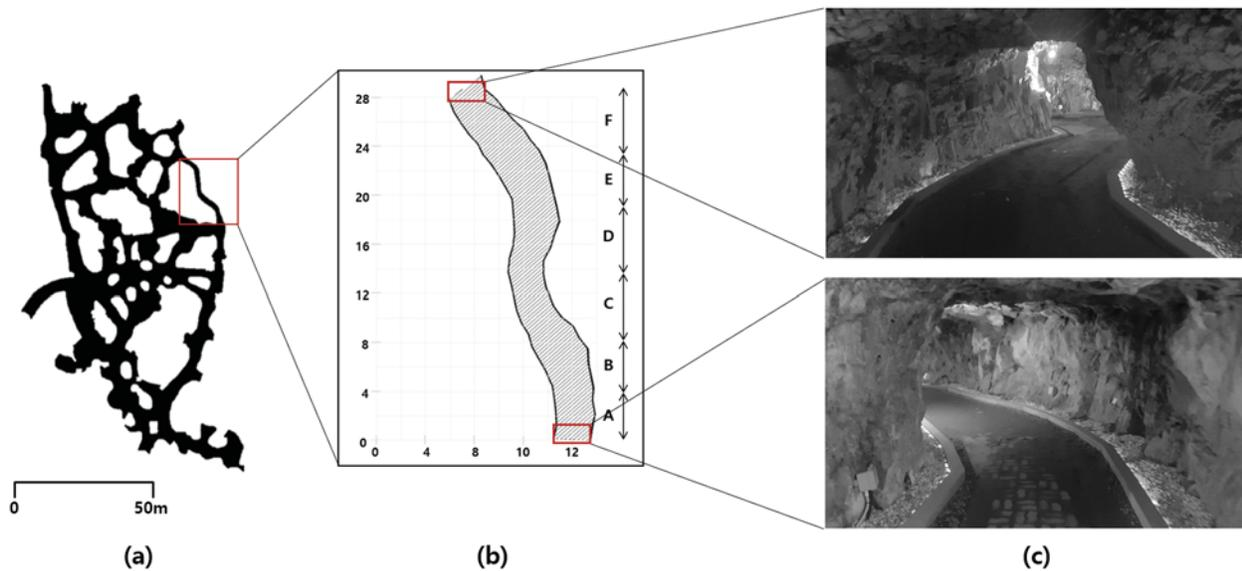
Figure 12: Conceptual diagram of the field experiment area (a) in an underground mine environment, (b) classified driving section, and (c) the start and end points
