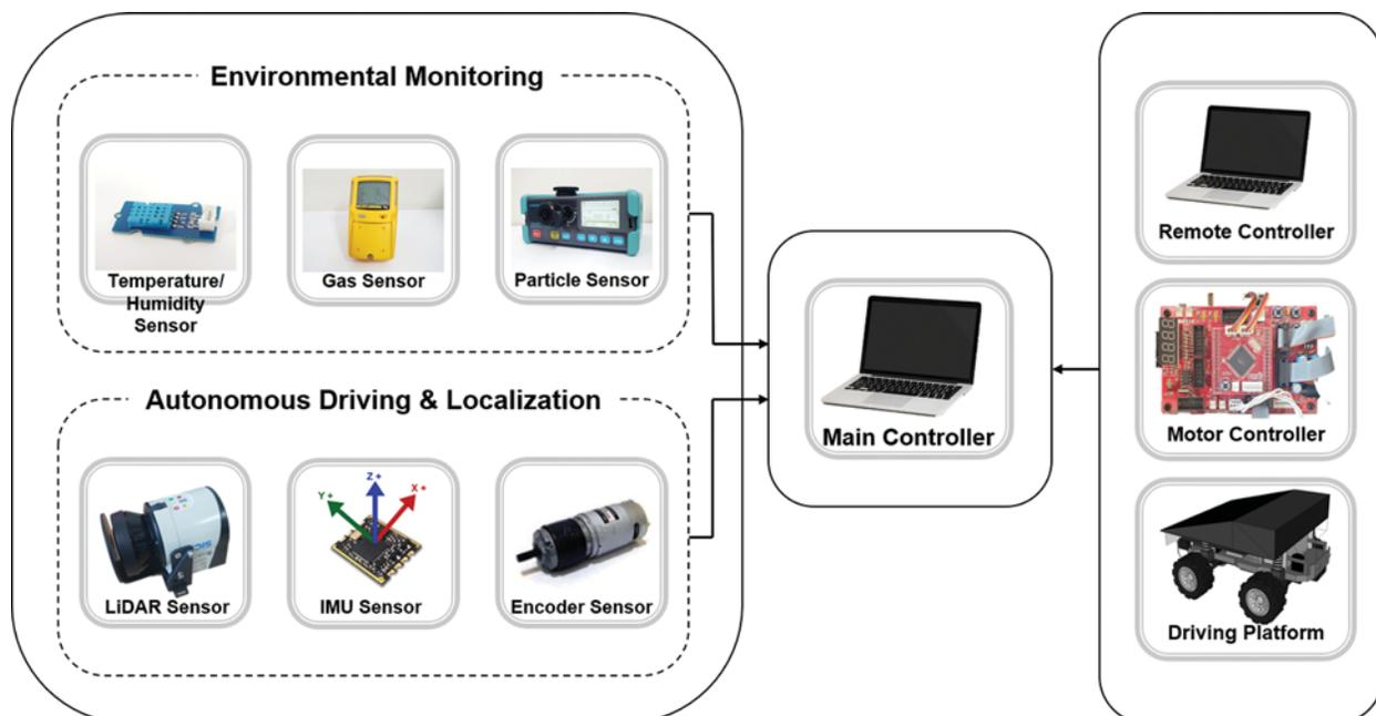
**Figure 1:** Overall structure of autonomous driving robot developed in this study
