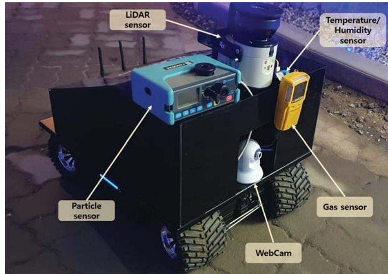
**Figure 2:** View of autonomous driving robot and sensors used in this study
