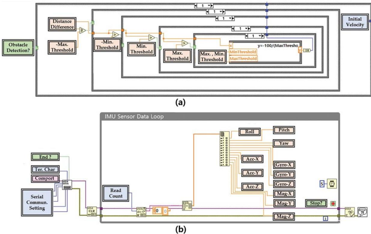
**Figure 10:** Block diagram of the programming code for (a) autonomous driving and (b) IMU sensor data acquisition
