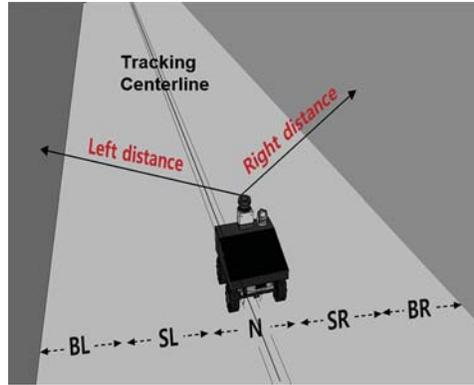
**Figure 6:** Conceptual diagram of the robot's driving states determined by the difference between distances to the left and right walls
