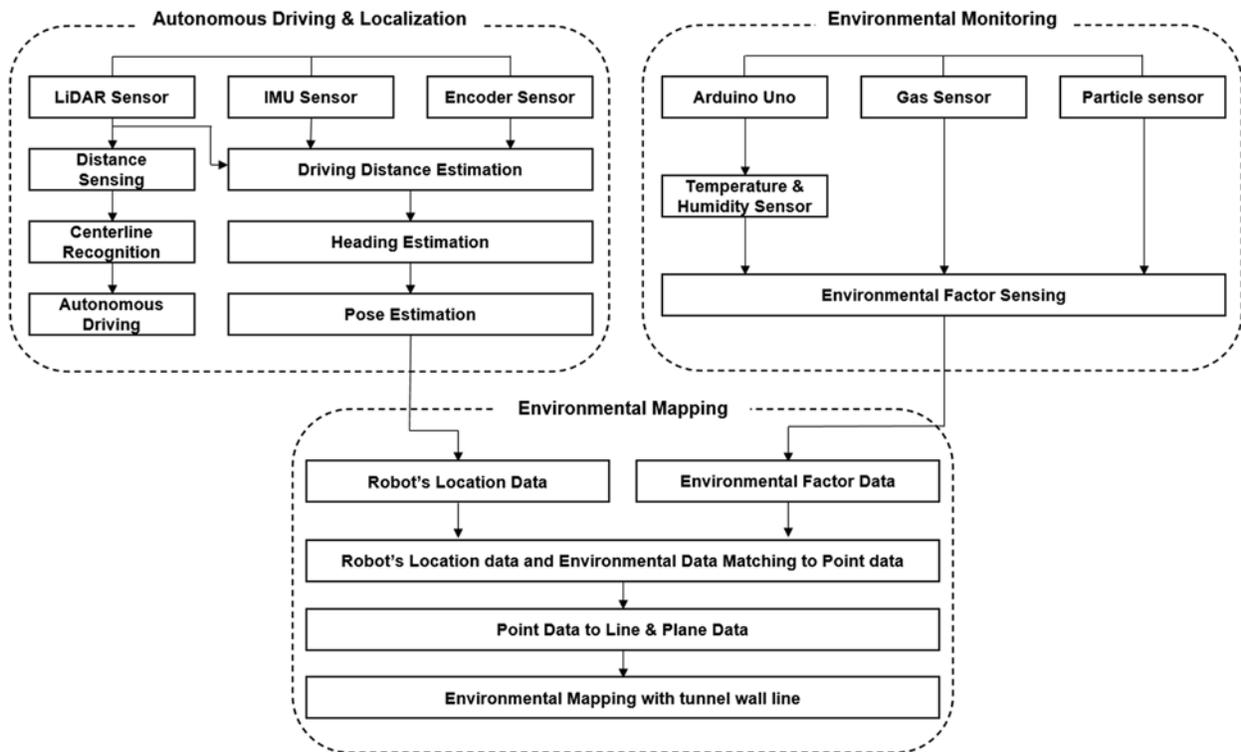
**Figure 4:** System architecture of environmental mapping system developed in this study
