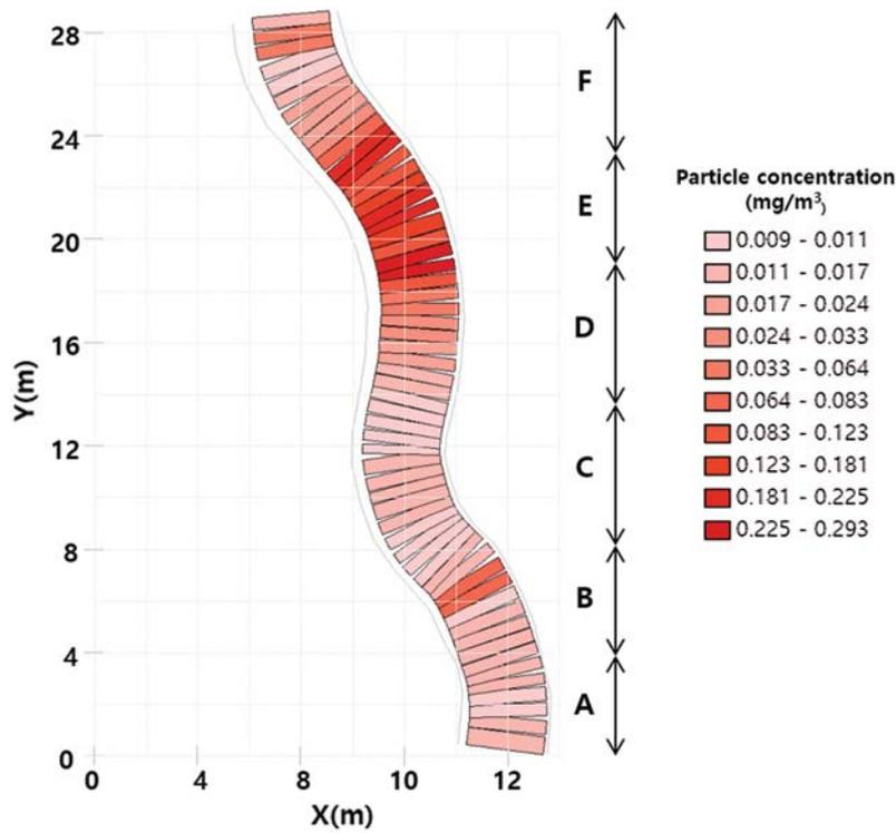
**Figure 16:** Particle concentration map at the study area created using the measured data and GIS
