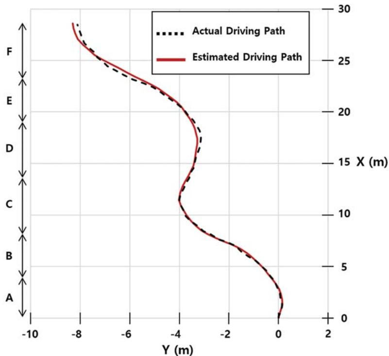
**Figure 15:** Comparison of the driving path created by the autonomous driving robot's location estimation method and the actual driving path
