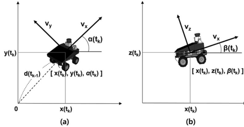
**Figure 7:** Dynamic model of the autonomous driving robot used in this study in the (a) xy-plane and (b) xz-plane
