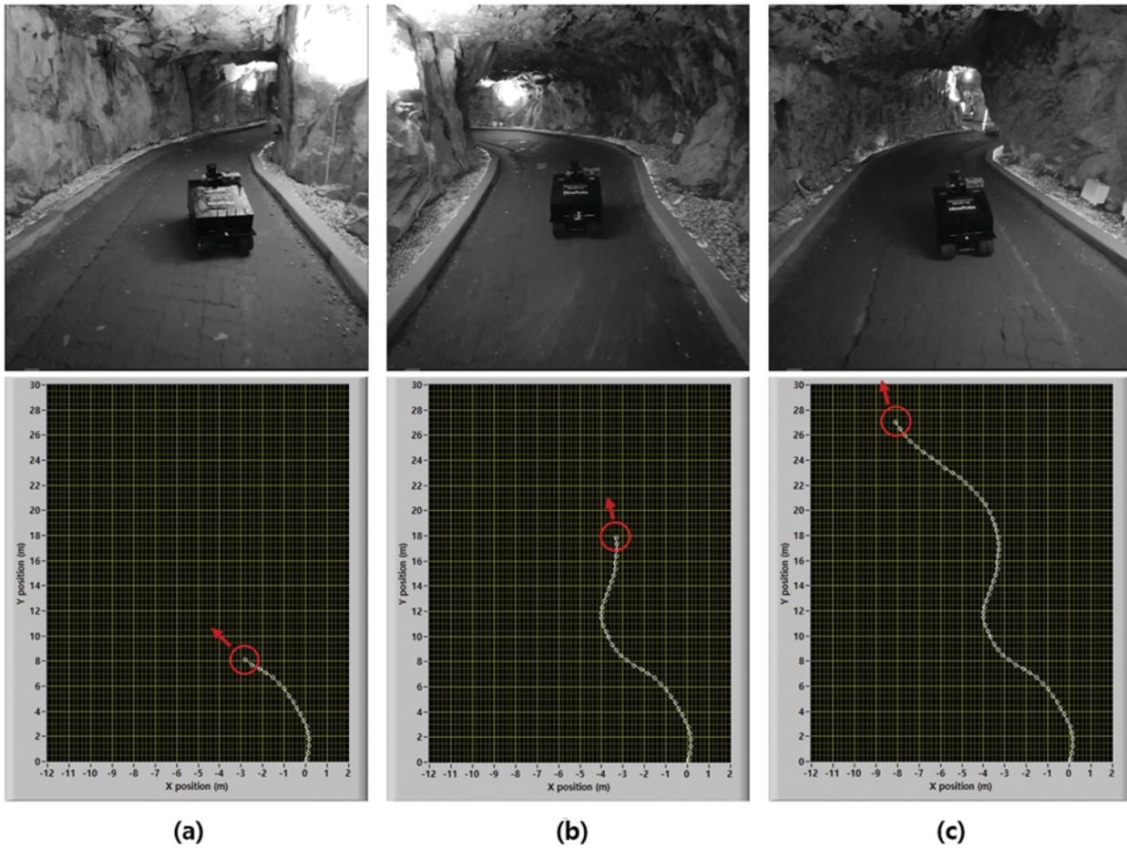
**Figure 13:** Field experiment scenes and estimated driving path of the autonomous driving robot at (a) 20 s (b) 40 s, and (c) 60 s
