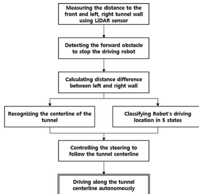
**Figure 5:** Procedure for controlling the autonomous driving robot's steering and stop functions in underground mines
