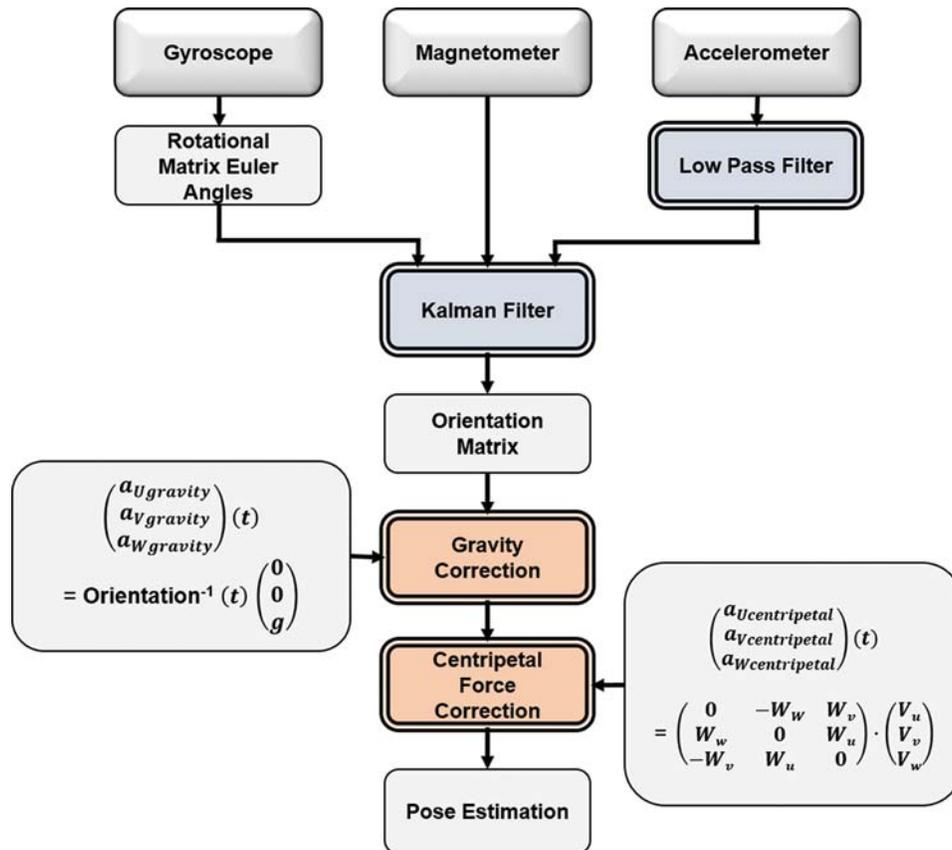
**Figure 9:** Processing diagram of IMU sensor's data to estimate the robot's pose and location
