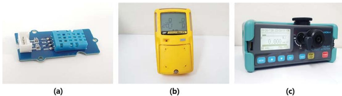
**Figure 3:** Environmental sensors used in this study. (a) Temperature & humidity sensor, (b) Gas sensor, (c) Particle sensor
