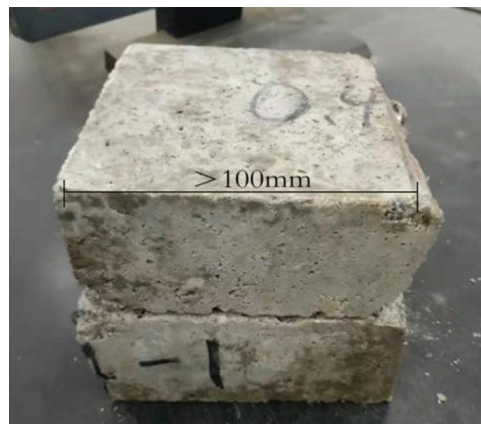
Figure 5: Compressive strength test-block
