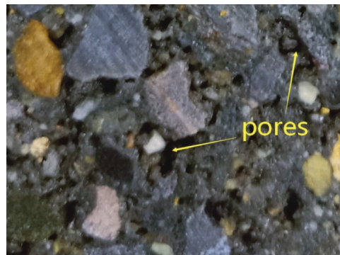
Figure 12: Baking-free brick slice images
