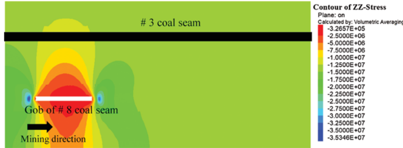
Figure 11: Vertical stress contours along the face advance direction in the PTCS for 30 m PVCS face advance
