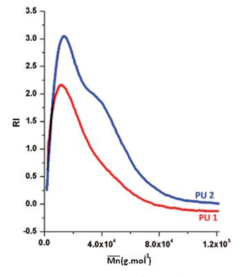
Figure 8: GPC curves of PU1 and PU2
