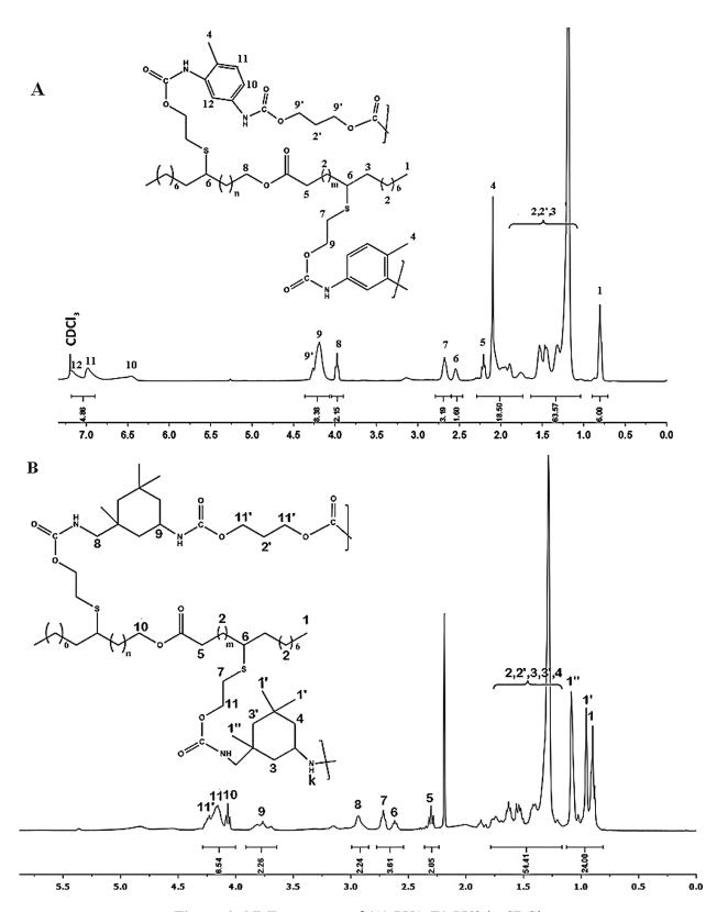
Figure 6: NMR spectrum of (A) PU1 (B) PU2 in CDCl<sub>3</sub>
