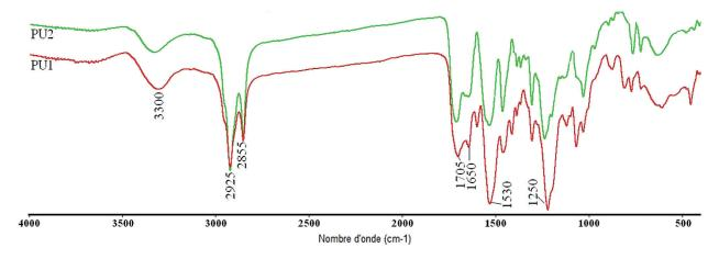
Figure 5: FTIR spectrum of PU1 and PU2
