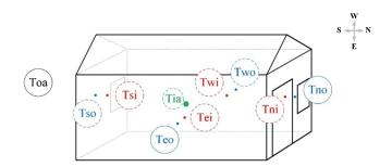
Figure 3: Distribution of T-type thermocouple probes in DTH
