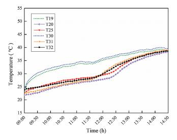
Figure 9: Temperature profiles of PCMs and indoor air (Position 1: With distance of 200 mm)
