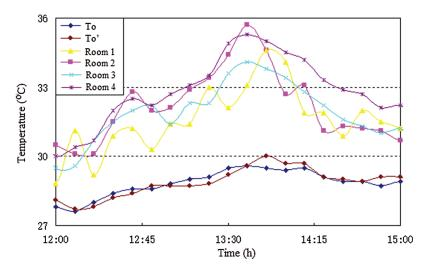
Figure 5: The difference between outdoor air temperature and air temperature inside DTHs
