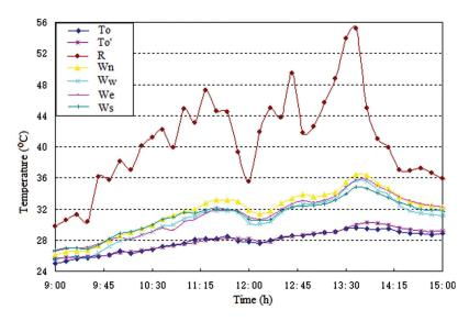
Figure 6: The difference between outdoor air temperature and inner surface temperatures of DTHs
