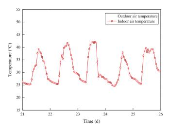
Figure 7: Comparison of outdoor air temperature and air temperature inside DTH in summer
