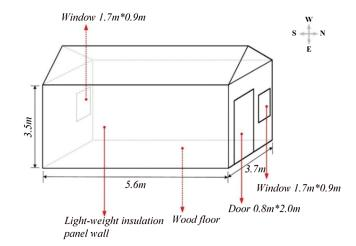
Figure 1: Illustration of experimental DTH. Adapted with permission from [22]. Copyright © 2018, Elsevier
