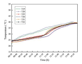
Figure 11: Temperature profiles of PCMs and indoor air (Position 3: With distance of 5 mm)
