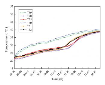
Figure 10: Temperature profiles of PCMs and indoor air (Position 2: With distance of 100 mm)
