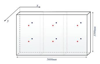
Figure 4: Distribution of T-type thermocouple probes in PAS
