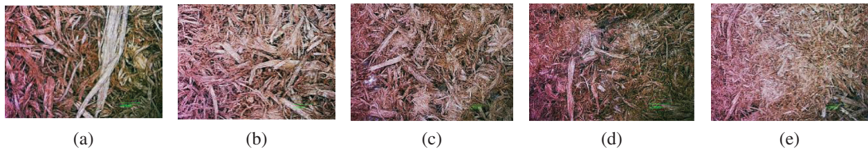
Figure 3: Poplar fiber under steam explosion pressure of 3.0 MPa. (a) 120 s, (b) 140 s, (c) 160 s, (d) 180 s, (e) 200 s
