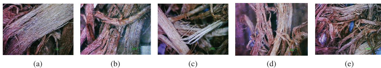
Figure 1: Poplar fiber under steam explosion pressure of 2.0 MPa. (a) 120 s, (b) 140 s, (c) 160 s, (d) 180 s, (e) 200 s
