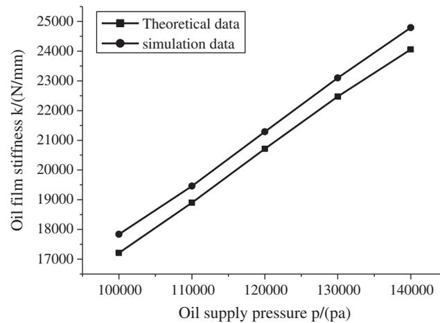
**Figure 12:** Correlation between oil supply pressure and oil film stiffness of the hydrostatic guide
