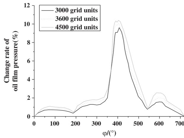
**Figure 5:** Effect of grid density on oil film pressure
