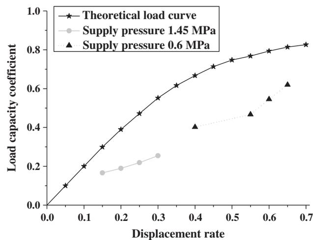
**Figure 13:** Experimental curve and theoretical curve of the dimensionless bearing capacity coefficient
