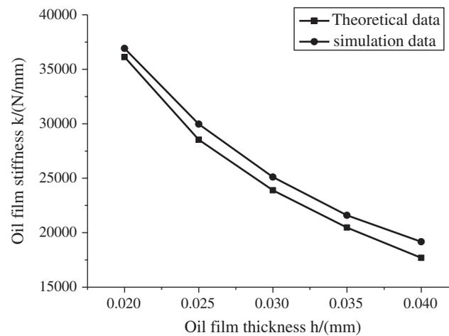
**Figure 11:** Oil film stiffness curve with different oil film thickness
