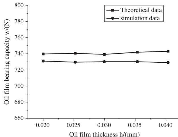
**Figure 8:** Bearing capacity at different film thicknesses
