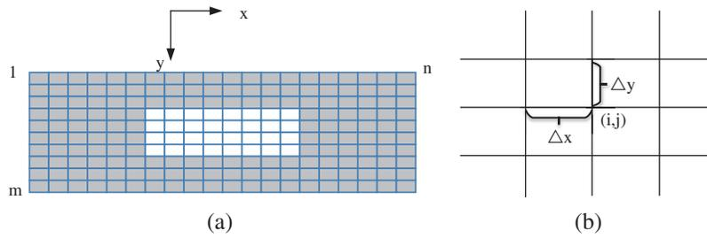
**Figure 2:** Finite difference discrete grid of a rectangular oil film. a) Discrete grid. b) Node data search
