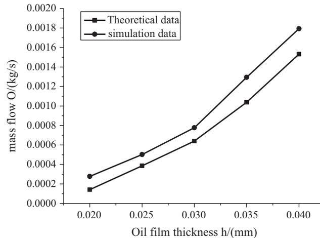
**Figure 9:** Mass flow rate of oil inlet with different oil film thickness
