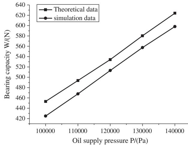
**Figure 10:** Correlation between oil supply pressure and oil film bearing capacity
