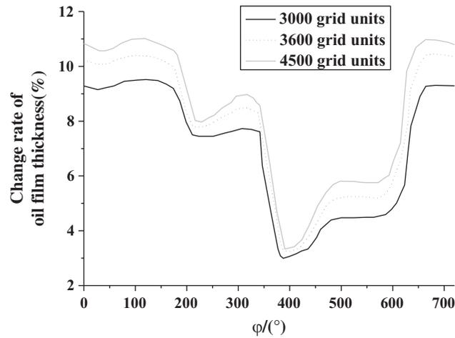
**Figure 7:** Impact of grid density on oil film thickness
