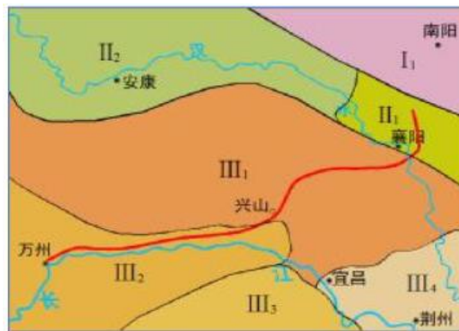
Figure 2: Strata distribution along Zhengwan high-speed railway route. (Figure: I formation of north China area, I 1 north Qinling partitions, II formation in Qinling area, II 1 basin south duct partition, II 2 south Qinling partition, III Yangzi stratum area, III 1 Dabashan mountain–Jingshan partition, partition III 2 Sichuan basin, III 3 Bamian mountain partition, partition III 4 Jiangnan basin.)
