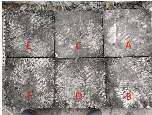
Figure 8: SSRAM specimens with different contents of steel slag placed outdoors for temperature measurements: (A) 0%, (B) 20%, (C) 40%, (D) 60%, (E) 80%, (F) 100%
