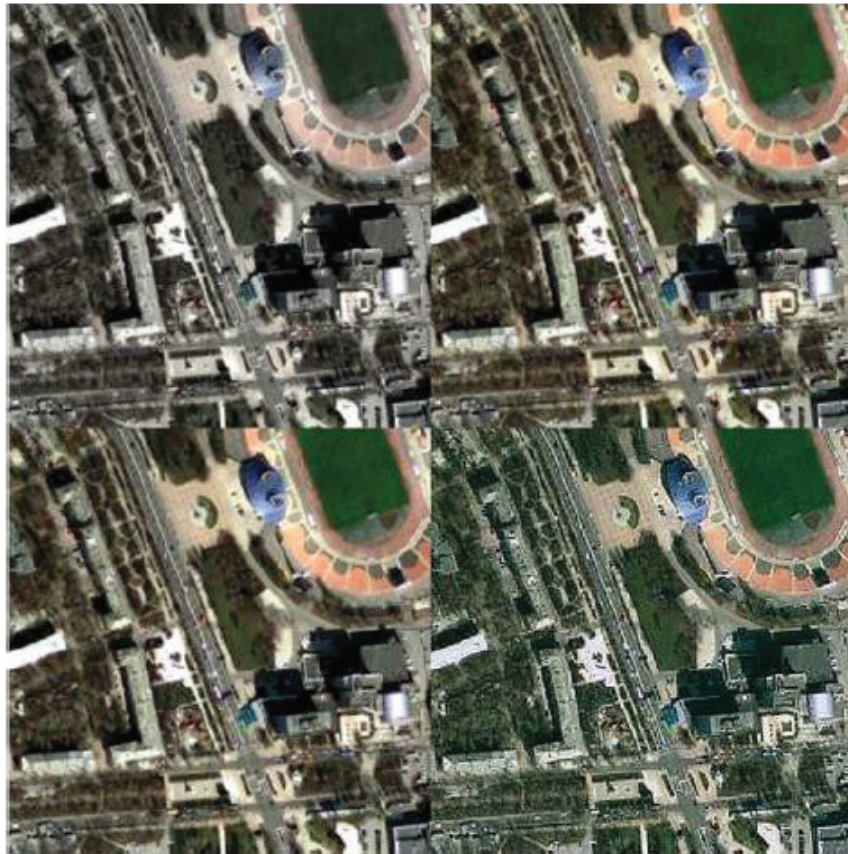
Figure 5 Result of image fusion (from left to right and from top to bottom - WA, IHS, HDWT, and DDWT).
