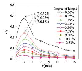
Figure 12: The effect of icing degree on wind energy utilization coefficient
