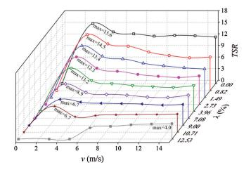
Figure 10: The effect of icing degree on TSR at different wind speeds
