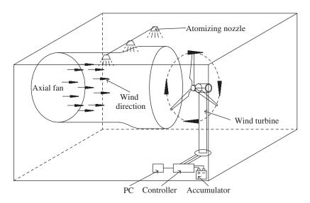
Figure 1: Schematic diagram of wind turbine blade icing test system
