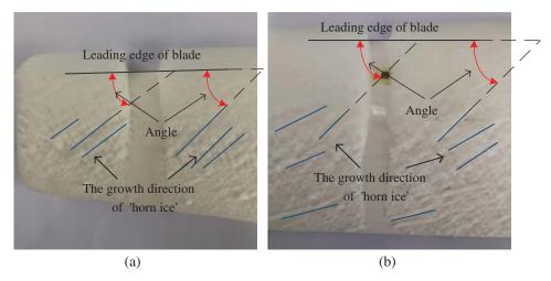
Figure 5: Glaze ice attached to the 0.95R and 0.6R leaves. (a) 0.95R icing state. (b) 0.6R icing state
