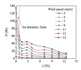
Figure 11: The effect of icing degree on output power
