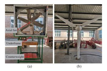
Figure 2: Wind turbine blade icing test device. (a) Axial fan. (b) Wind turbine
