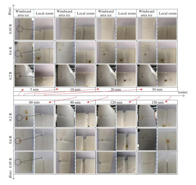
Figure 4: Blade icing test results
