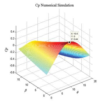
Figure 13: Numerical simulation results of  $C_P$
