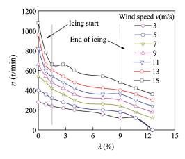
Figure 9: The effect of icing degree on rotating speed
