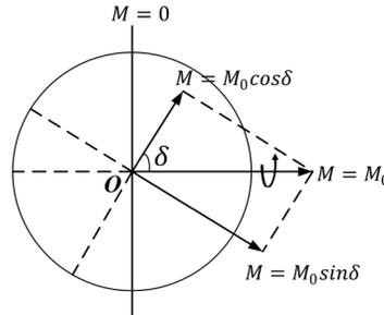
**Figure 3:** Torque decomposition
