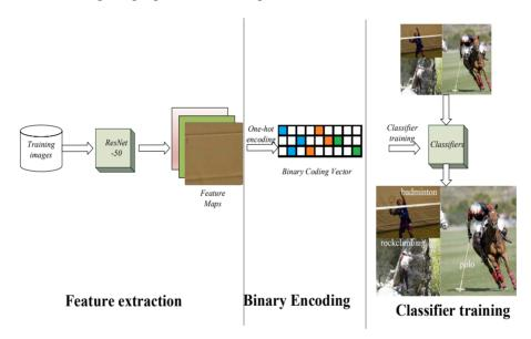
**Figure 1:** The framework of our proposed method, which consists of three stages: A) Feature extraction B) Binary encoding and C) Classifier training
