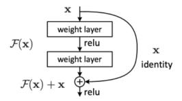
Figure 4: The residual block of ResNet [He, Zhang, Ren et al. (2016)]
