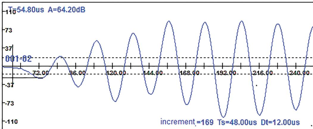
Figure 6: Received waveforms of defect-free concrete
