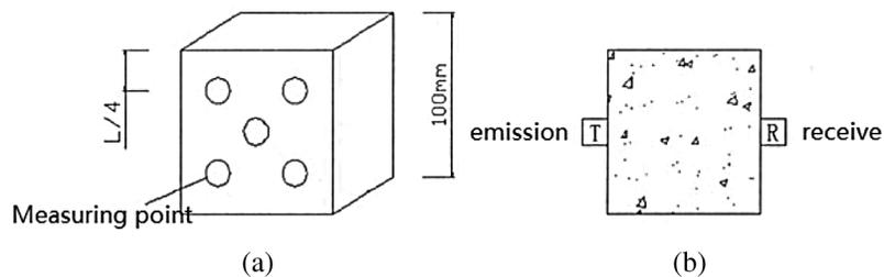
**Figure 3:** Measuring point layout
