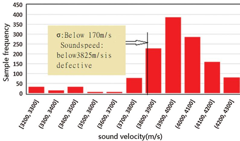
**Figure 9:** Distribution of sound speed in all columns
