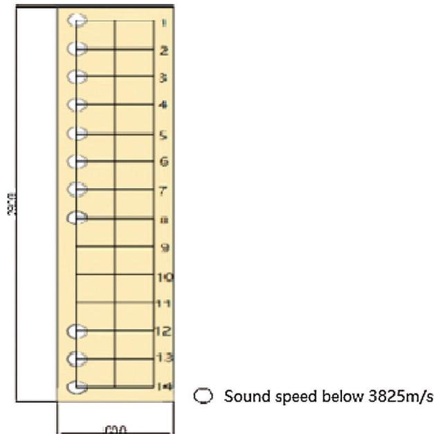
Figure 12: Pillar B test result diagram
