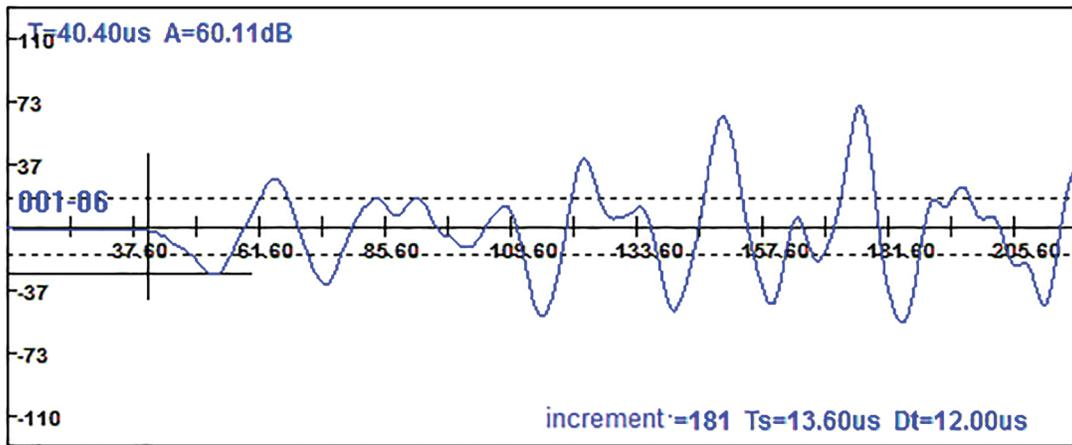
Figure 7: Received waveforms of defective concrete
