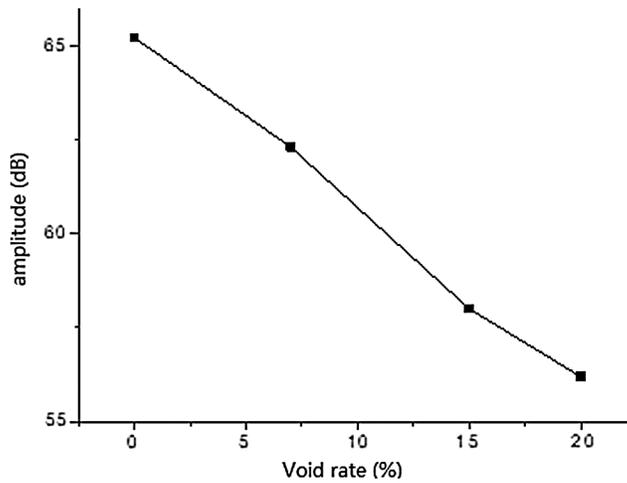
Figure 8: Curves of the variation of the amplitude of the specimens with different emptying rates
