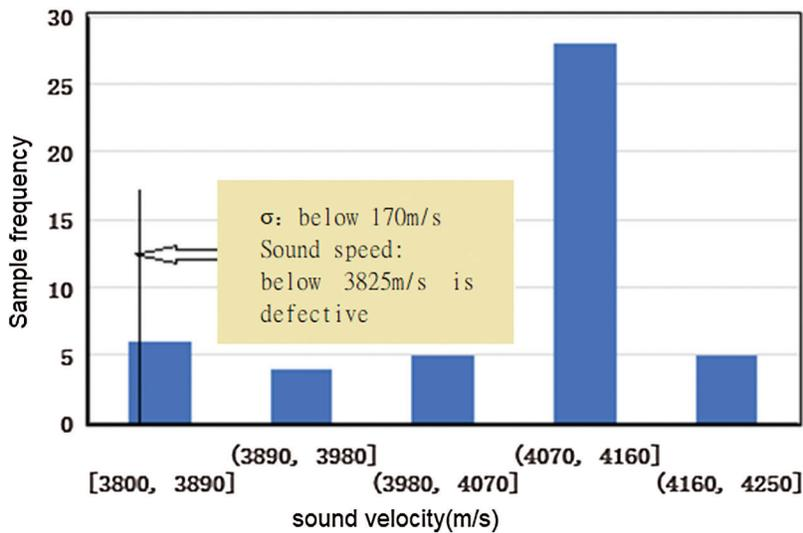
**Figure 10:** Sound velocity distribution of column part A
