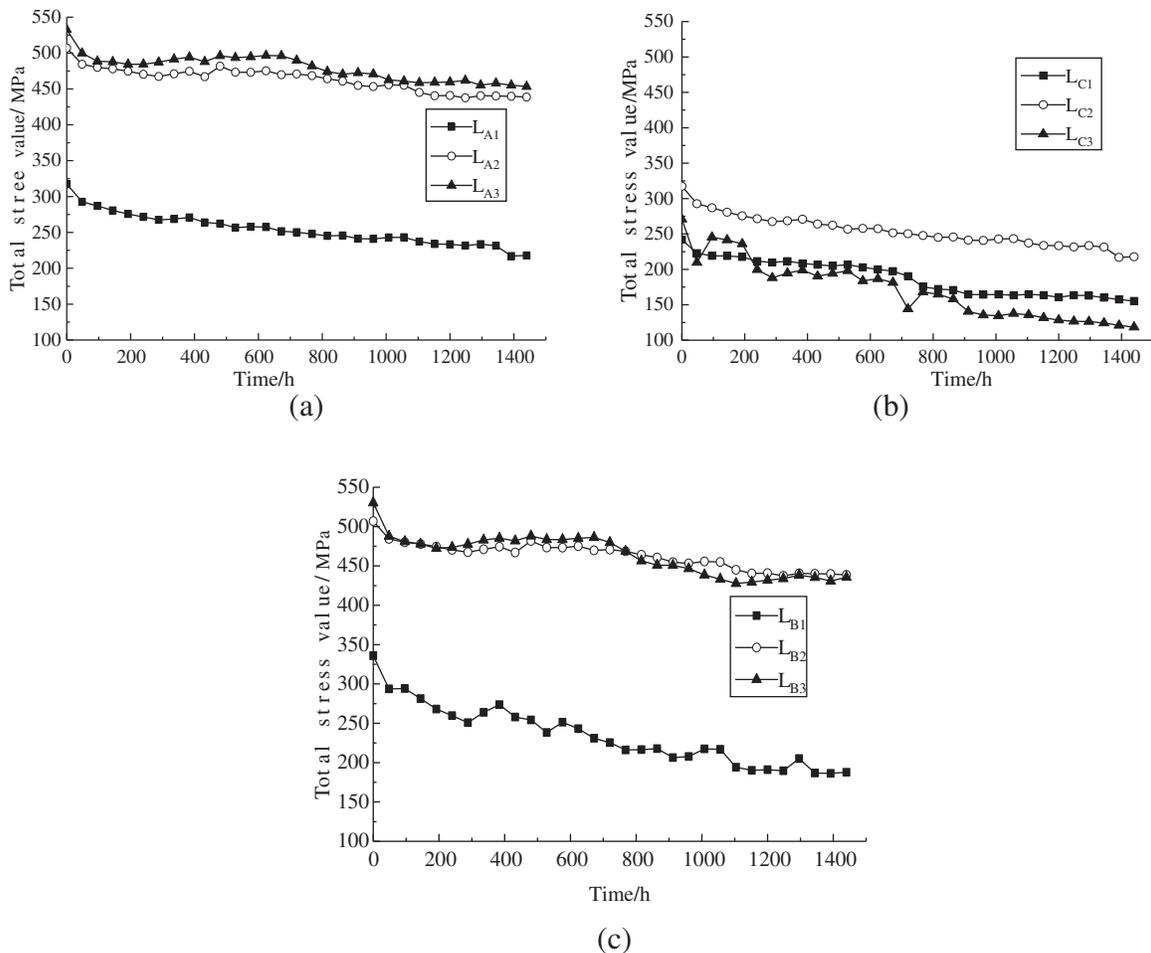
**Figure 7:** Change curve of total steel wire stress with time. (a) Group A, (b) Group B and (c) Group C
