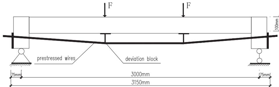
**Figure 12:** The schematic diagram of the prestressed glued bamboo and wood beam
