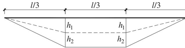
**Figure 16:** Overall calculation sketch of the pre-stressed GBWB
