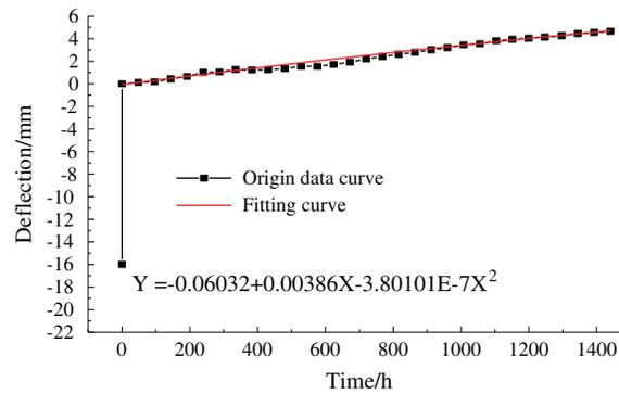
**Figure 11:** Fitting curve of the total deflection on the  $L_{A1}$  beam midspan with time
