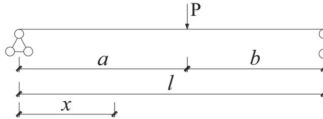
**Figure 13:** The schematic diagram of the concentrated force
