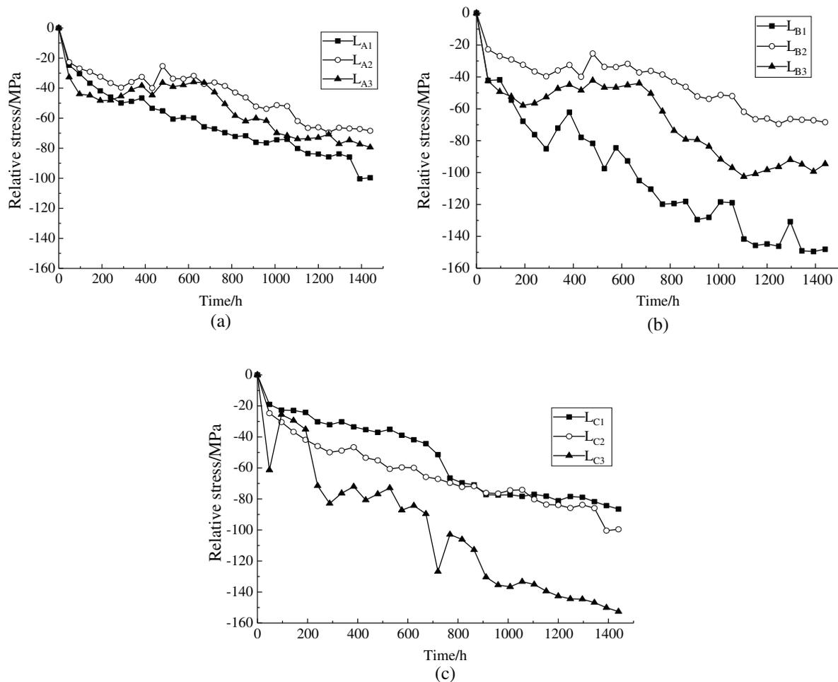
**Figure 8:** Change curve of relative stress of steel wire with time. (a) Group A, (b) Group B and (c) Group C
