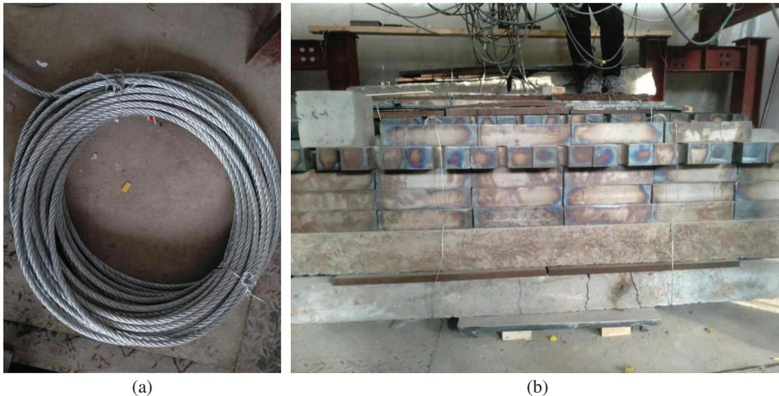
**Figure 3:** Long-term test loading. (a) Steel cable and (b) Weight and tray
