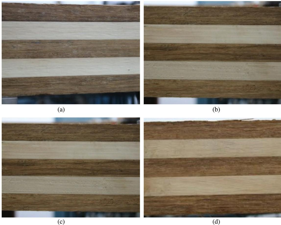
**Figure 6:** State diagram of pre-stressed GBWB during long-term test. (a) Test start, (b) The 20<sup>th</sup> day, (c) The 40<sup>th</sup> day and (d) The 60<sup>th</sup> day
