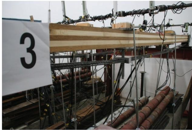
**Figure 5:** Picture of Long-term test loading
