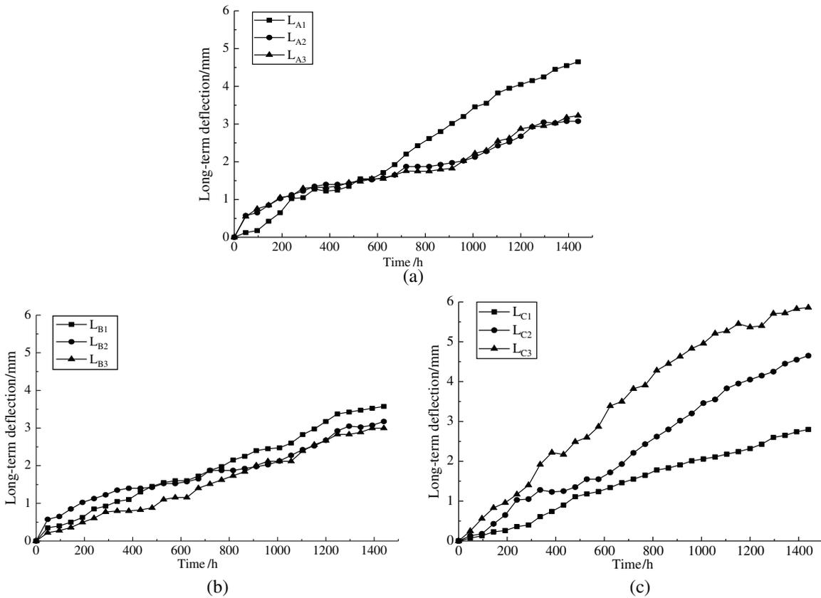
**Figure 10:** Change curve of the long-term deflection of the beam midspan with time. (a) Group A, (b) Group B and (c) Group C
