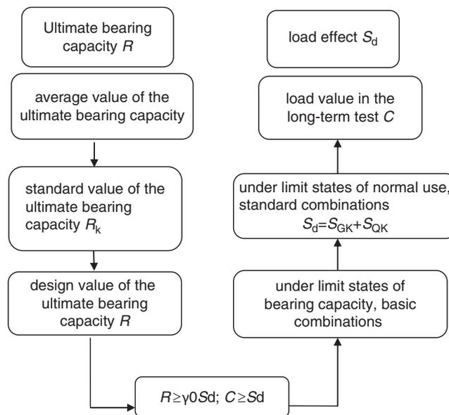
**Figure 4:** The derivation flowchart of the load value in the long-term loading test
