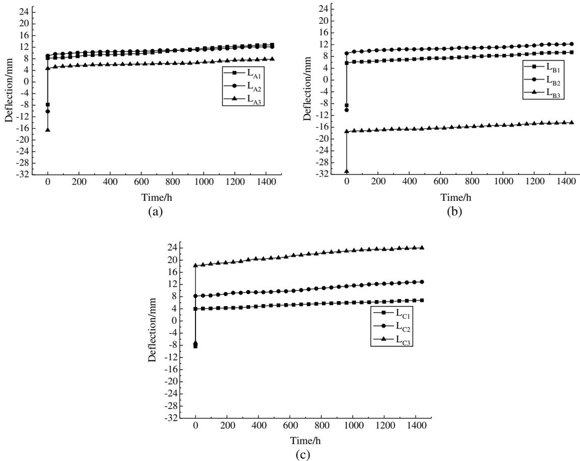
**Figure 9:** Change curve of total deflection on beam midspan with the time. (a) Group A, (b) Group B and (c) Group C
