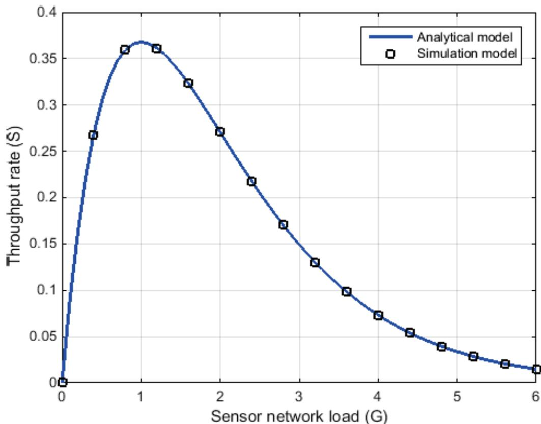
Figure 3 Slotted Aloha technique throughput rate
