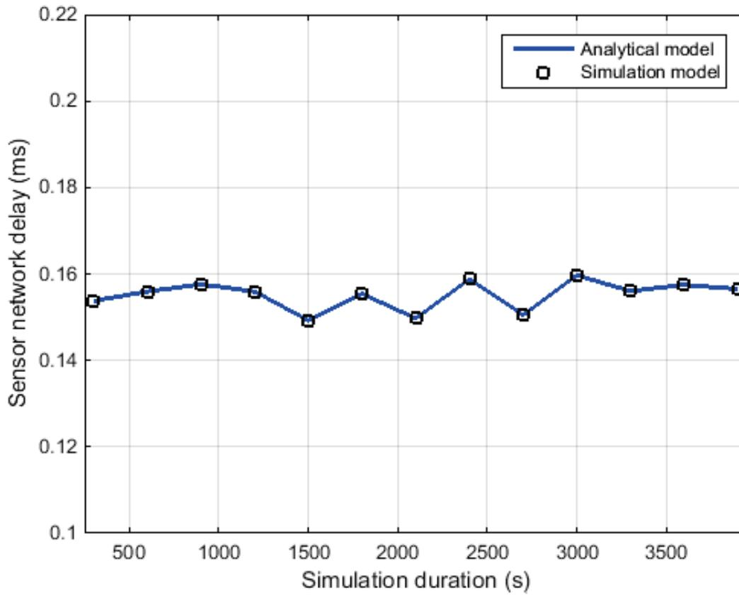
Figure 4 Slotted Aloha technique delay analysis
