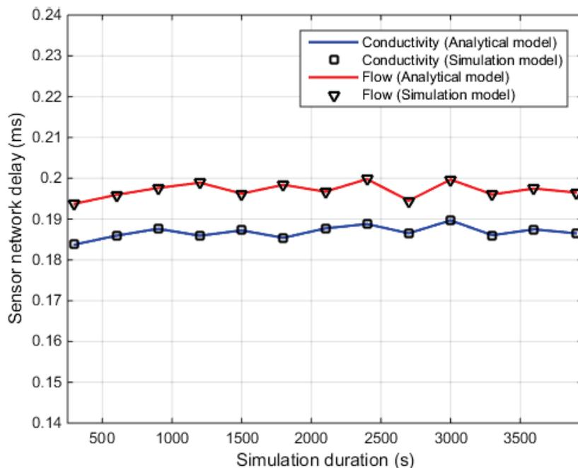
Figure 10 Delay analysis for low priority classes
