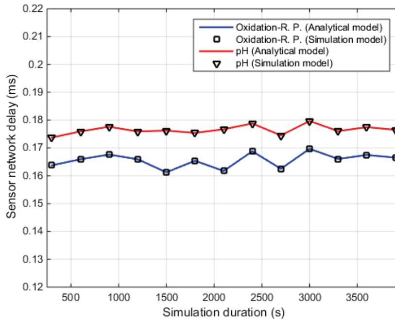
Figure 9 Delay analysis for high priority classes
