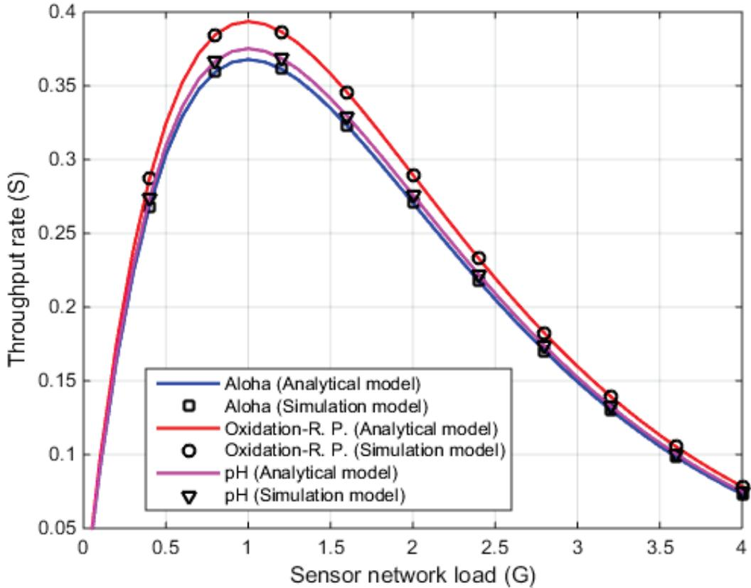
Figure 7 Throughput for high priority classes with double data rate
