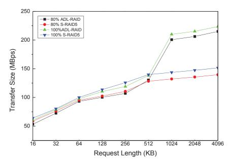
Figure 6 The comparison of the transfer size between ADL-RAID and S-RAID5.
