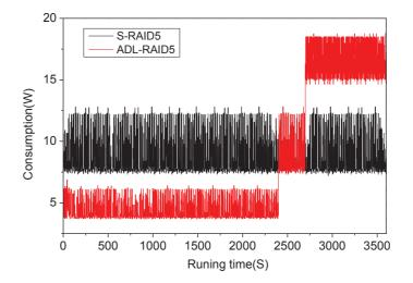
Figure 9 The comparison of the energy consumption of S-RAID5 and ADL-RAID.
