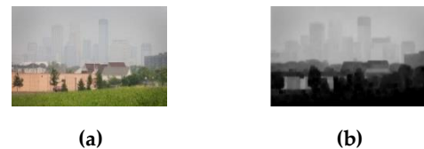
Figure 5. (a) Hazy image, and (b) dark channel of (a). (The originally input is from http://dinosauriens.info/?u=Air++Minnesota+Pollution+Control+Agency )
