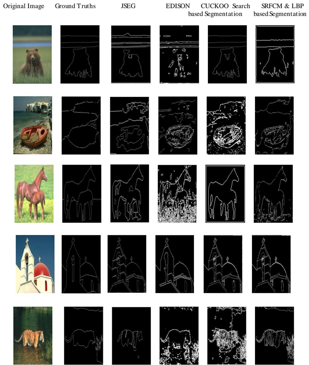
**Figure 5.** Comparison of segmentation results obtained by the proposed algorithm SRFCM & LBP with state of the art algorithms
