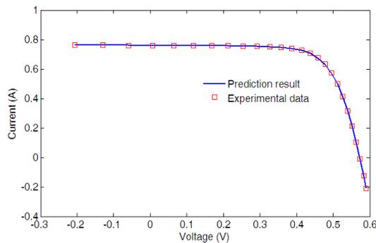
Figure 2. Prediction results of the double diode model
