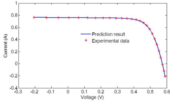
Figure 1. Prediction results of the single diode model
