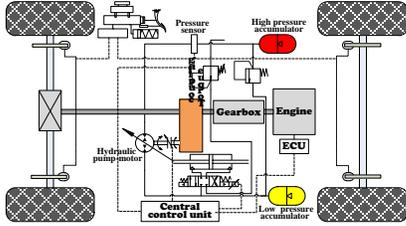
Figure 1. Structure Diagram of RPHHV.
