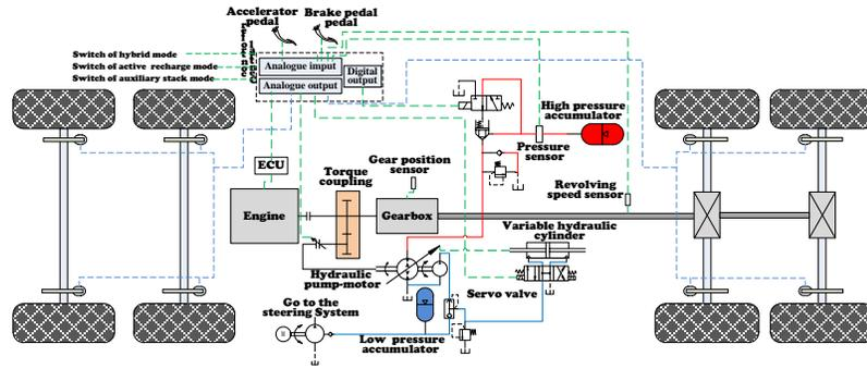
Figure 14. The Structure Diagram of the FPHC Experimental Prototype.
