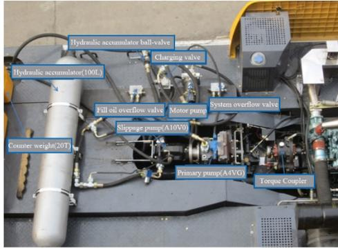
**Figure 13. Hydraulic Hybrid System Diagram of the FPHHC Experimental Prototype.**
