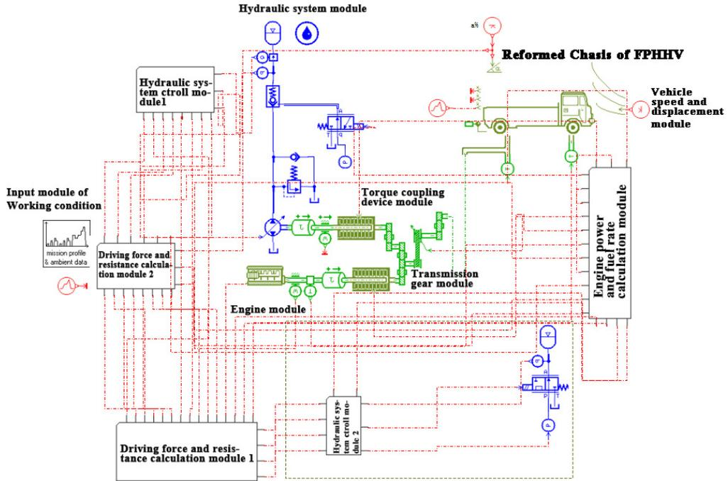
Figure 3. Simulation Model of the FPHC Based on AMESim.
