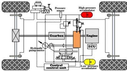
Figure 2. Structure Diagram of FPHHV.
