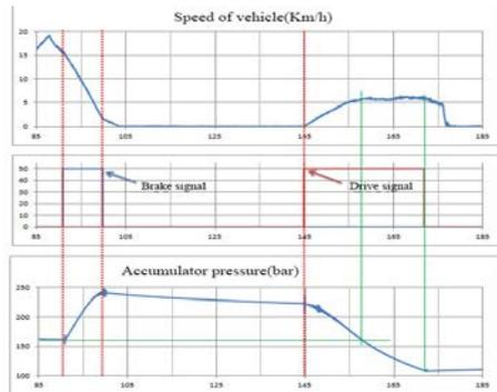
Figure 16. System Parameter Changes in the Process of Energy Utilization.
