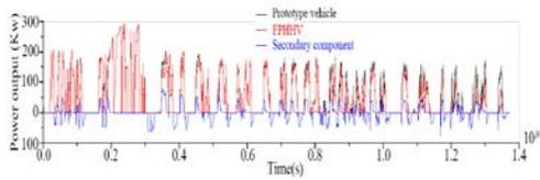
**Figure 7.** Power Output of the Engine and the Secondary Component.
