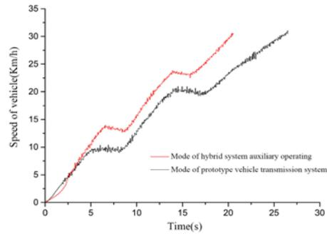
Figure 17. Speed Curves of the Vehicle is Accelerated from Idle State to the Speed of 30 Km/h.
