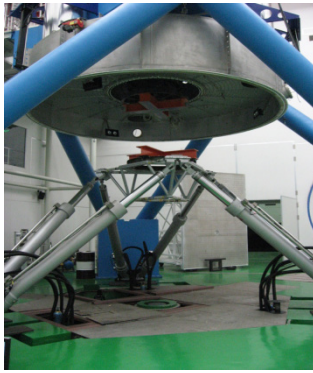
Figure 1. The Parallel Manipulator Constructed for the Space Docking Motion Simulation.
