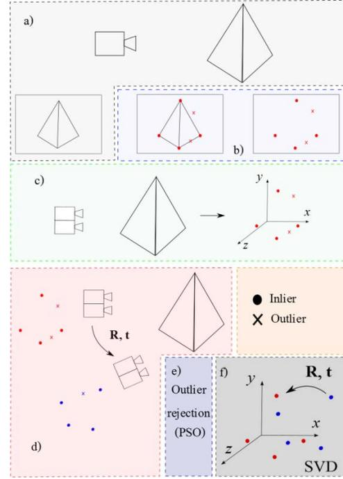
**Figure 3. Diagram of the algorithm. a) Image capture. b) Feature extraction. c) 3D information obtained with stereo vision. d) Two sets of points, due to cameras movement. e) Outlier rejection with PSO. f) Pose estimation with SVD.**
