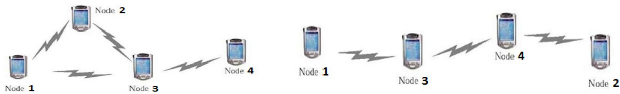
Figure 13. The Effect of Local Node Mobility. Tasks Executing on Nodes 1 and 2 Communicate Directly. During the Execution of a Task, Node 2 moves within the Network Coverage Area and therefore is not Directly Accessible to Node 1. Thus, a Task Executing on Node 1 Communicates with a Task Executing on Node 2 through Two Intermediate Nodes, i.e., Nodes 3 and 4. This Increases the Data Transfer Time and, thus, the Task Completion Time.
