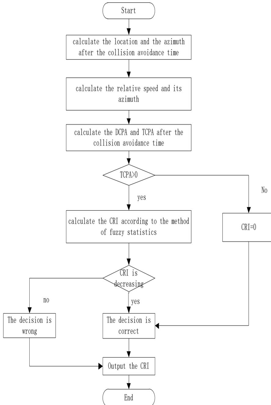
**Figure 5** The CRI after collision avoidance
