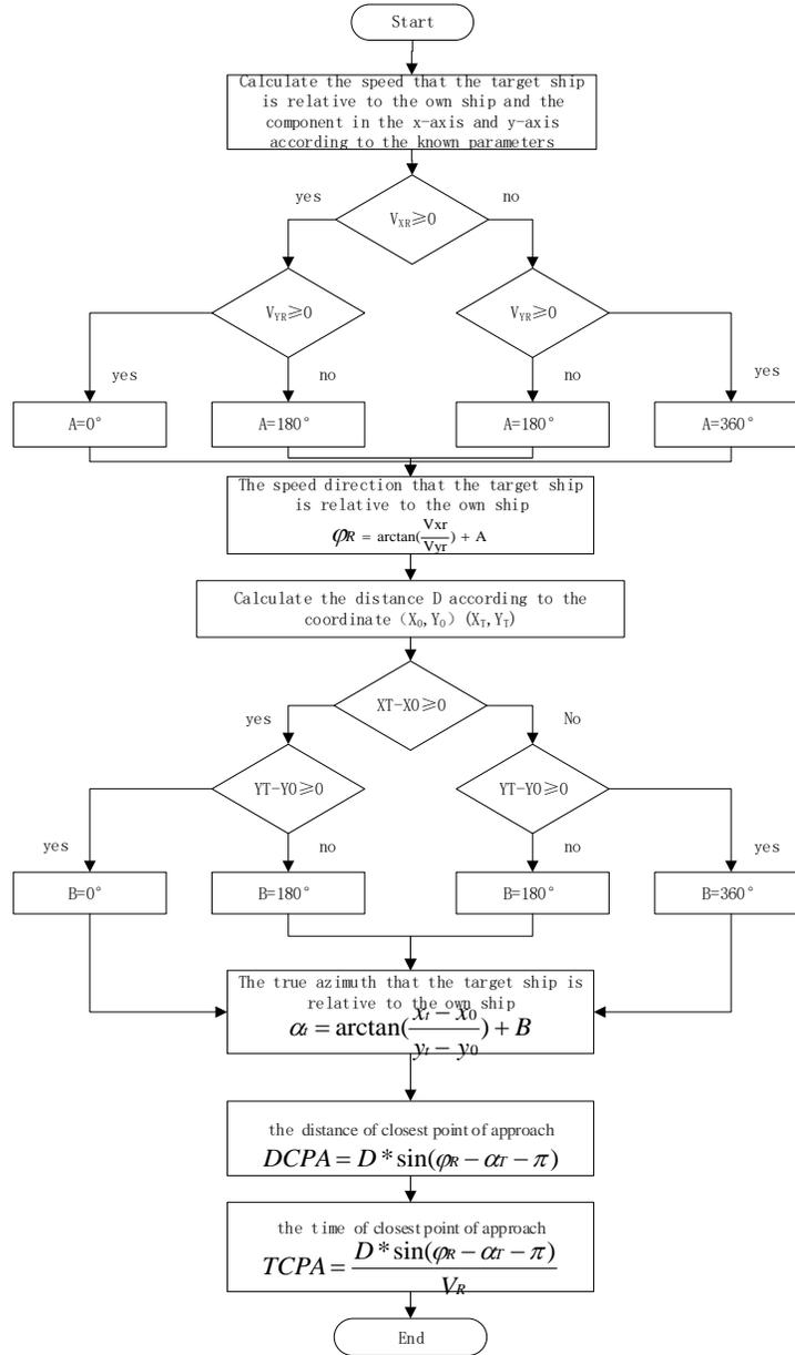
**Figure 1** the realize the process of DCPA and TCPA Set own vessel at the initial position  $(x_0, y_0)$ , speed  $V_0$ , heading for  $\varphi_0$ , collision avoidance angle  $\Delta\varphi$ ; target ship  $(x_t, y_t)$ , speed is  $V_t$ , heading for  $\varphi_t$ . Then:
