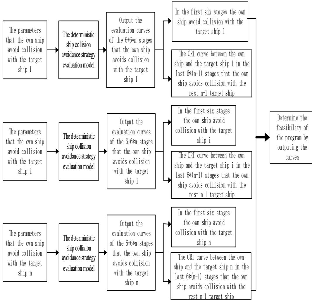
Figure 11 the diagram of feasibility assessment for multi-vessels collision avoidance scheme
