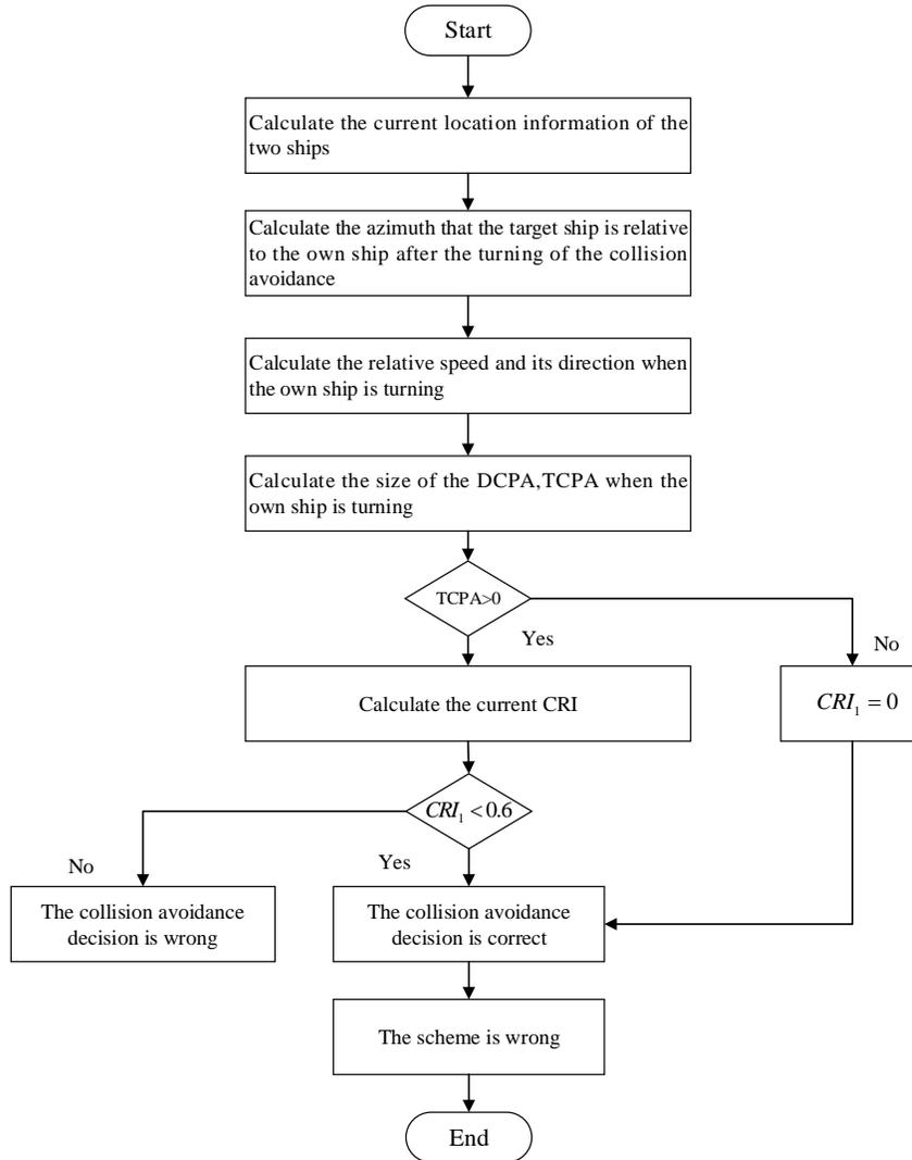
Figure 4 The CRI before collision avoidance
