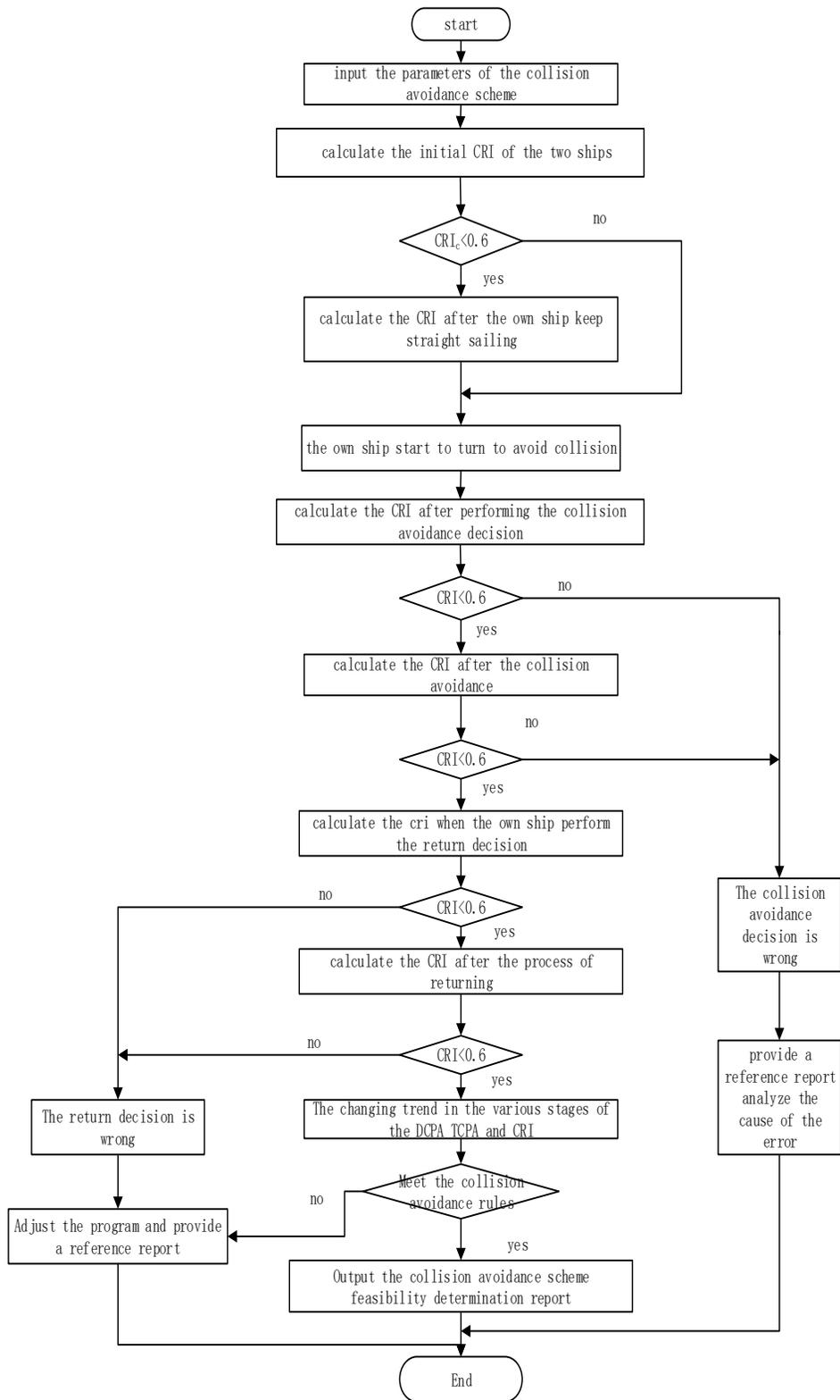
Figure 7 Vessel collision avoidance scheme feasibility Analysis flow chart
