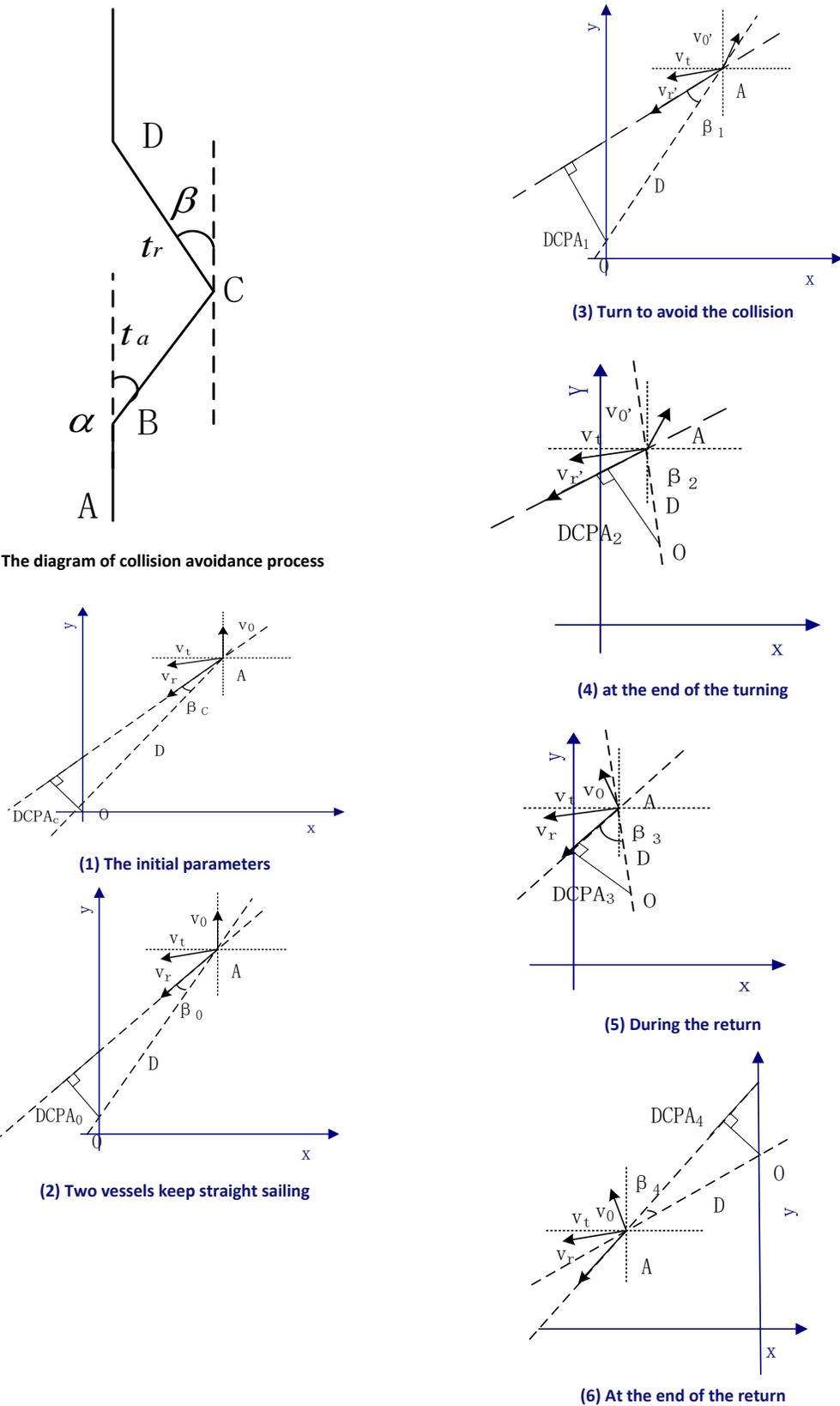
Figure 9 The stages schematic diagram of avoidance collision target vessel
