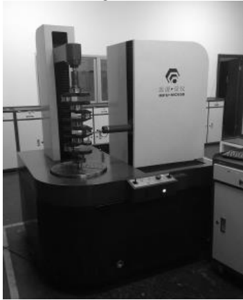
Figure 9. Tracking mode crankshaft measuring instrument based on four axis coordinated motion system
