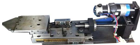
Figure 3. The structure of servo tracking probe
