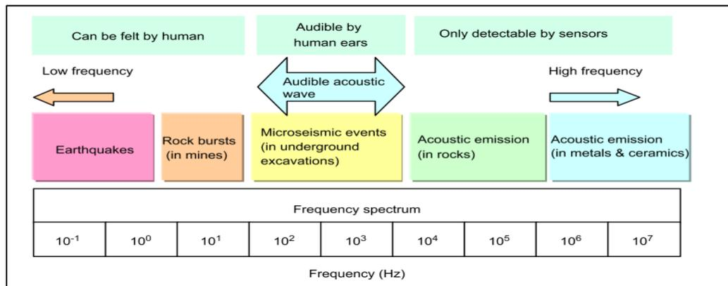
Figure 5. Acoustic emission frequency range and its applications.
