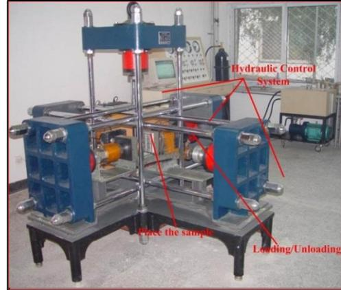
Figure 1. Three-axial rockburst experiment system.
