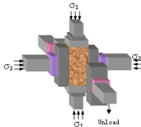
Figure 2. Sketch of the three-axial rockburst experiment system mechanism.
