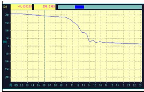
Figure 4. A typical vertical load curve of a granite rockburst.
