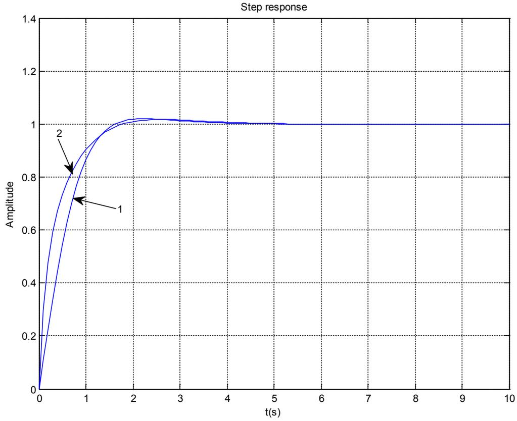
Fig. 5 Step response for  $G_2(s)$  using the proposed method and the existing method (Can & Ozguven, 2017).
