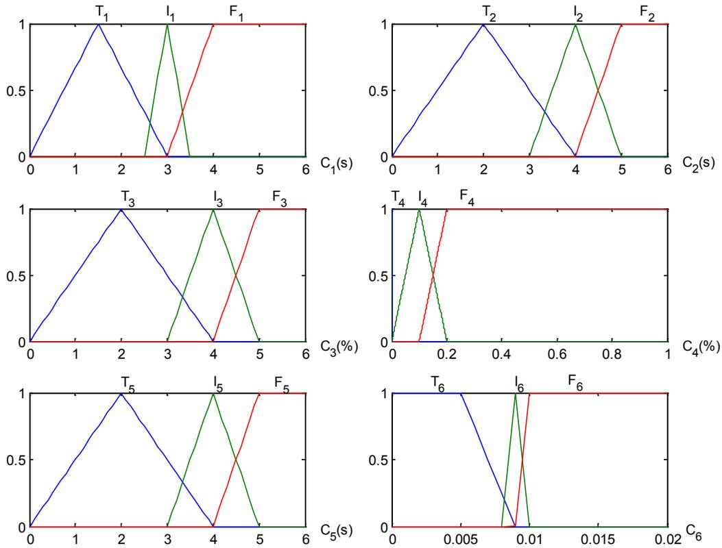
**Figure 2.** The membership functions of six transient state characteristics. C1: rising time (s), C2: settling time (s), C3: overshoot ratio (%), C4: undershoot ratio (%), C5: peak time (s), and C6: steady-state error.
