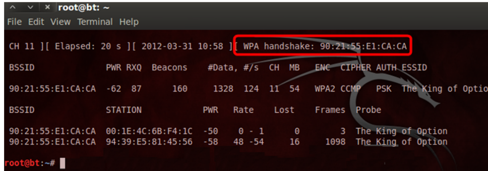
Figure 5. The capturing of the WPA handshake
