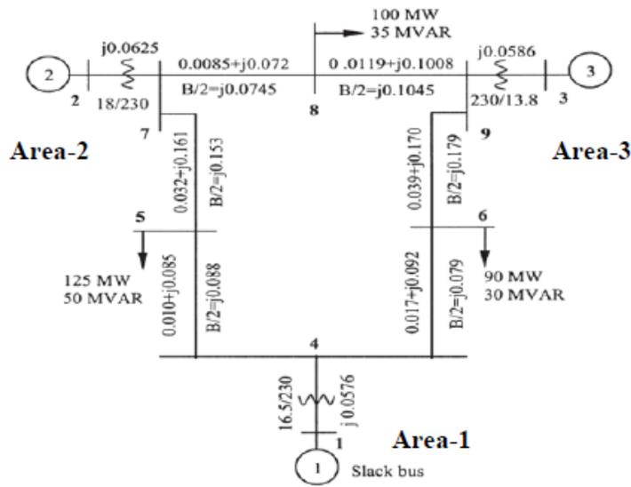
Figure 3. IEEE (WSCC) 3-machine, 9-bus Interconnected Power System Model.
