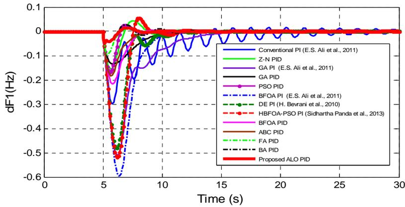
Figure 9. Frequency deviation in Area-1 for multi step load disturbances.
