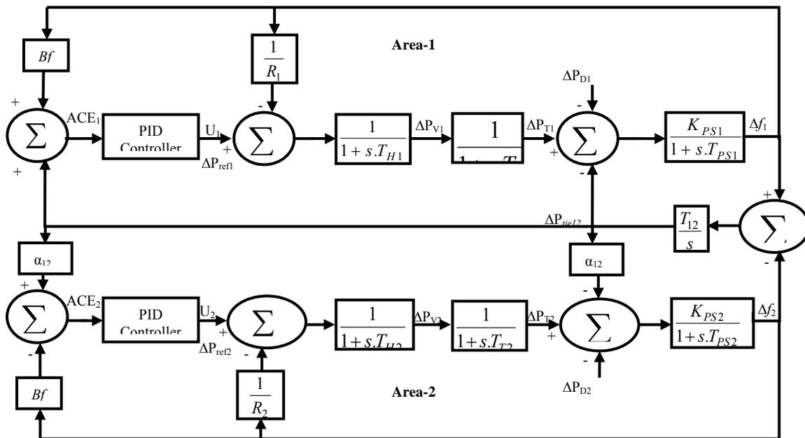
Figure 2. LFC model of Two-Area Interconnected Power System.
