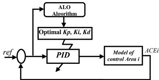
**Figure 7. Proposed ALO based PID controller model.**
