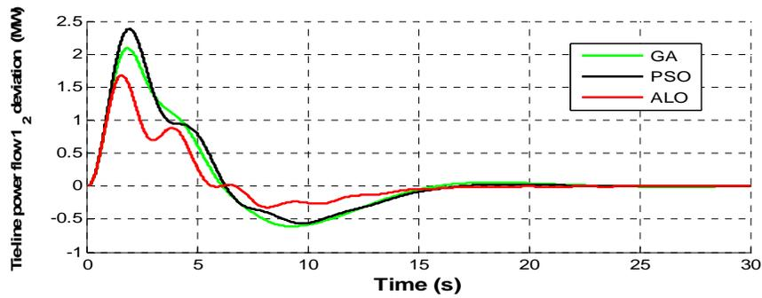
Figure 12. Tie-line power flow deviation between Area-1 and Area-2.
