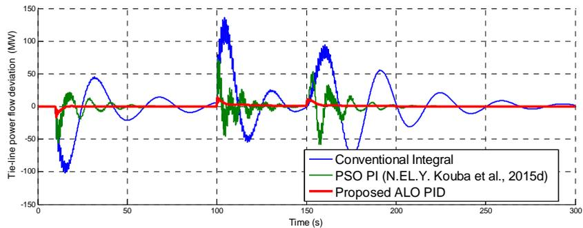
Figure 14. Tie-line power flow deviation  $\Delta P_{12}$  between Tunisia and Algeria.
