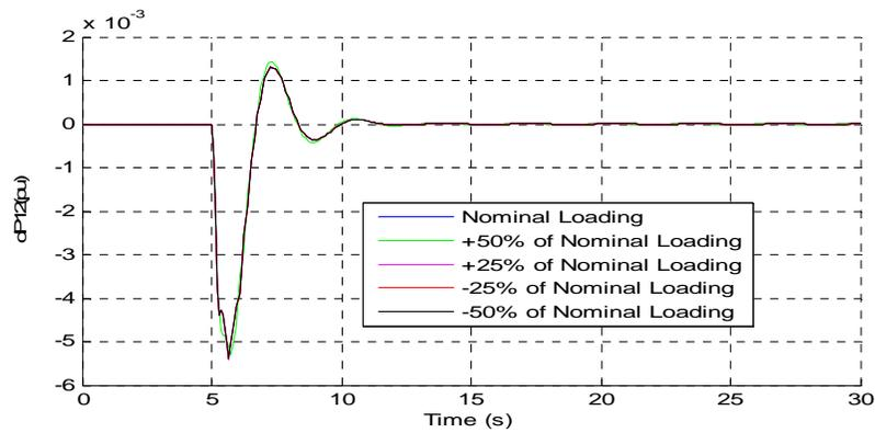
Figure 10. Change in tie-line power deviation with change in loading condition.
