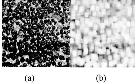
**Figure 7:** Background gray value calculated in the second time: (a) Image after illumination equalization and (b) Background gray values calculated from image
