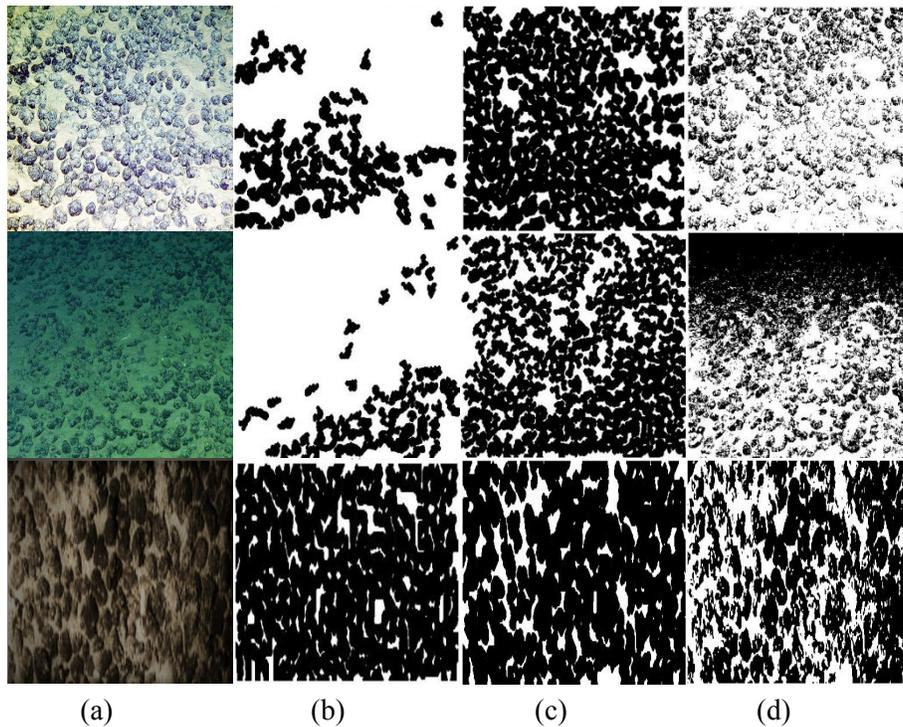
**Figure 12:** Result of image segmentation: (a) Original image; (b) Image segmentation results of unrepaired manganese nodules; (c) Result of image segmentation after processing by this method; (d) Result of binarization of original image
