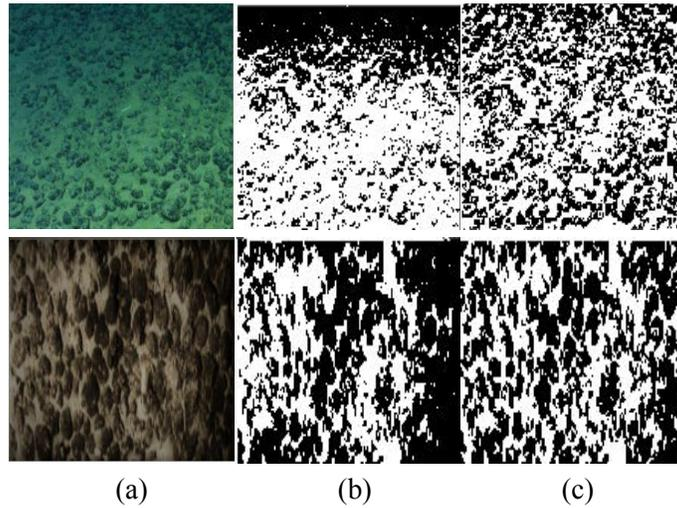
**Figure 13:** Segmentation results of Otsu: (a) Original image; (b) Segmentation results of uneven illumination image; (c) Segmentation results of uniform illumination image
