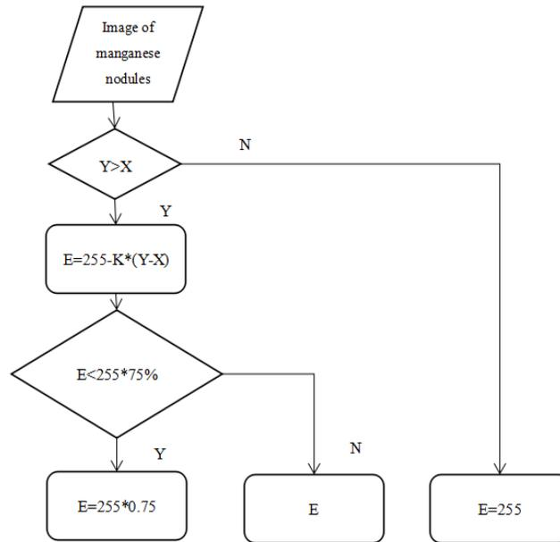
**Figure 5:** Contrast adjustment block diagram
