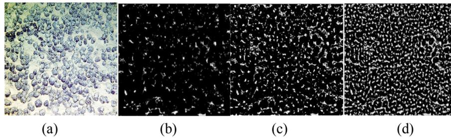
**Figure 9:** Effect of different masks on restoration: (a) Original image; (b) Overlarge mask; (c) Moderate mask; (d) Too small mask
