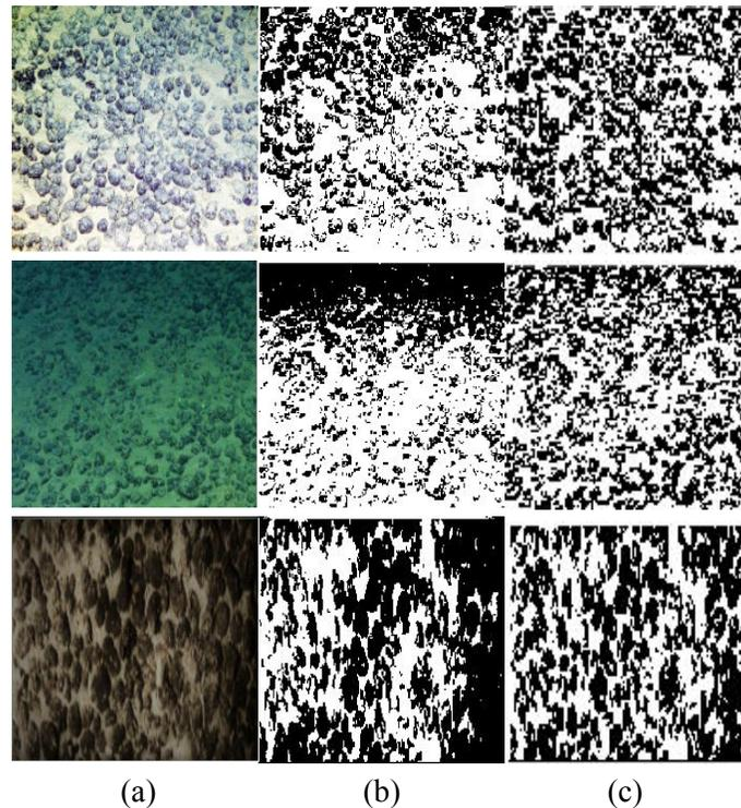
**Figure 15:** Segmentation results of Iterative threshold method: (a) Original image; (b) Segmentation results of uneven illumination image; (c) Segmentation results of uniform illumination image
