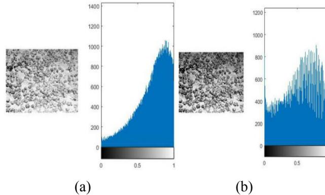
**Figure 3:** The gray histogram and image before and after grayscale stretching: (a) Before and (b) After
