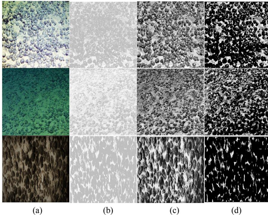
**Figure 6:** Result comparison of different methods: (a) Original image; (b) Processing results of original method; (c) Results of Retinex algorithm; (d) Processing results of this method
