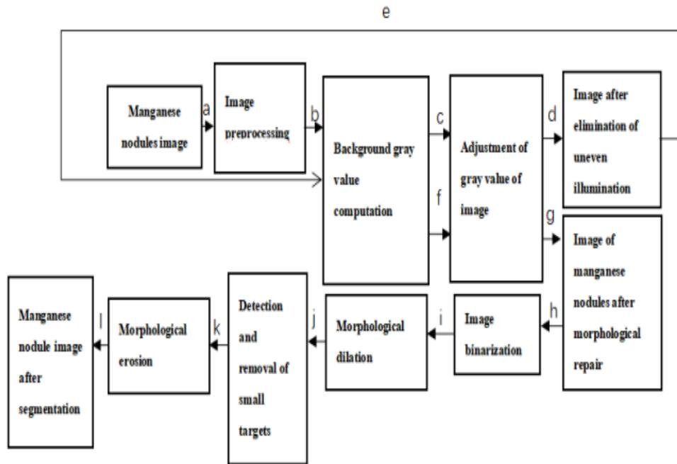
Figure 2: Flow chart of new method
