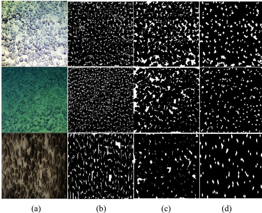
**Figure 8:** Comparison of different repair methods: (a) Original image of manganese nodules; (b) Repair results of this method; (c) Results in case (1); (d) Results in case (2)
