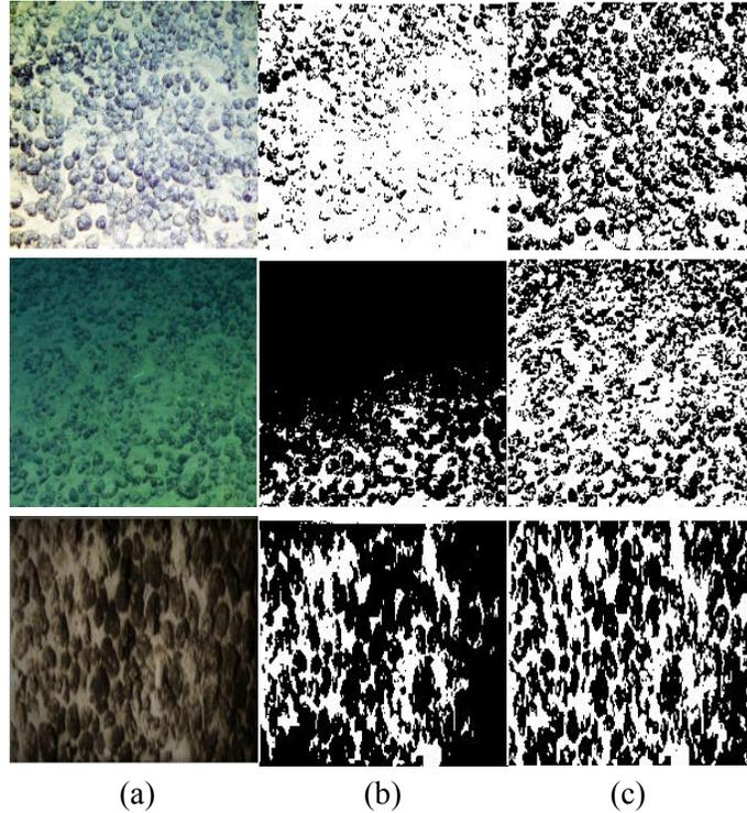
**Figure 14:** Segmentation results of maximum entropy method: (a) Original image; (b) Segmentation results of uneven illumination image; (c) Segmentation results of uniform illumination image
