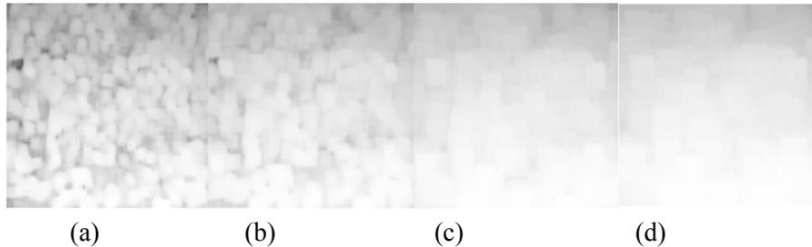
**Figure 4:** Background gray values calculated by masks of different sizes: (a)  $N=15$ ; (b)  $N=21$ ; (c)  $N=35$ ; (d)  $N=49$
