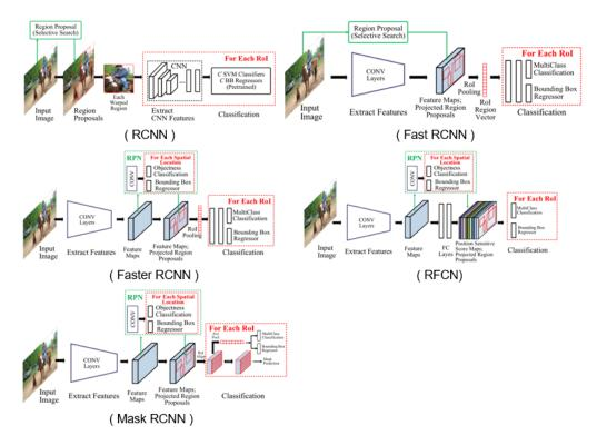
Figure 2: A brief description of several two-stage detector frameworks
