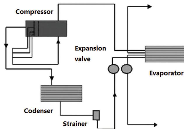
**Figure 3:** Working principle of air conditioning refrigerator
