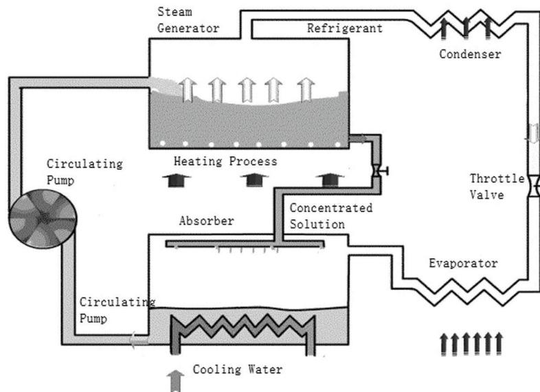
**Figure 1:** Working principle of HVAC
