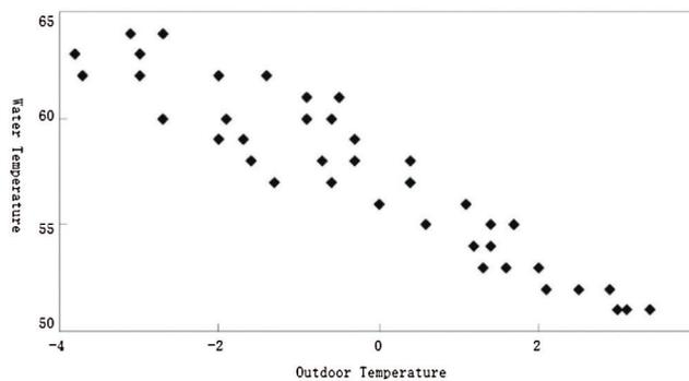
**Figure 2:** Scatter diagram of water supply temperature and outdoor temperature
