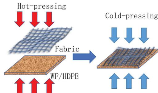
**Figure 1:** Preparation of a fabric-veneered wood fiber/high-density polyethylene (WF/HDPE) panel**Table 2:** Production parameters for veneering WF/HDPE board with the fabrics
