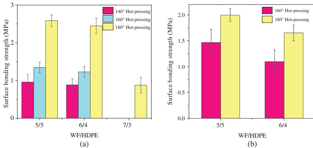
**Figure 3:** Bonding strength of wood fiber/high-density polyethylene (WF/HDPE) board covered by canvas fabric (a) or polyester fabric (b)
