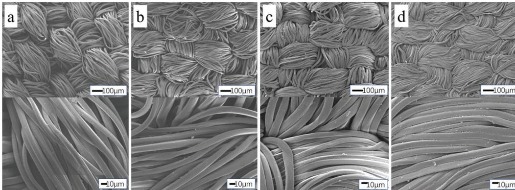
**Figure 5:** Electron microscopy studies at different magnifications of the fiber shape of a polyester surface under different hot-pressing temperature (WF:HDPE = 5:5, 6:4, 7:3): (a) unpressed; (b) hot pressed at 140°C; (c) hot pressed at 160°C; (d) hot pressed at 180°C
