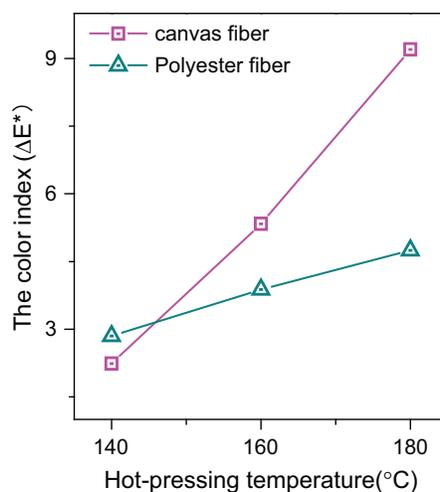
**Figure 6:** Color change in fabric at different hot-pressing temperatures
