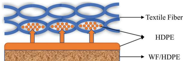
**Figure 9:** Adhesion mechanism between textile fabric fibers and WF/HDPE composite
