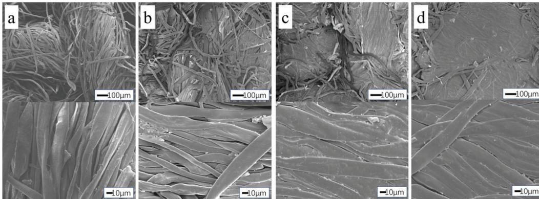
**Figure 4:** Electron microscopy studies at different magnifications of the fiber shape of a canvas surface under different hot-pressing temperature (WF:HDPE = 5:5, 6:4, 7:3): (a) unpressed; (b) hot pressed at 140°C; (c) hot pressed at 160°C; (d) hot pressed at 180°C
