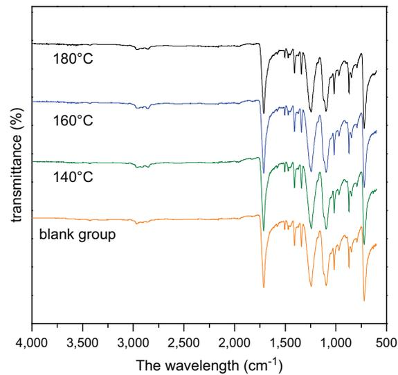
**Figure 8:** Infrared spectra of polyester fabric after hot pressing
