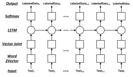
Figure 4: Schematic diagram of the LSTM model
