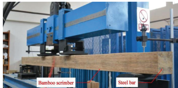
Figure 1: Newly designed reinforced bamboo scrimber composite (RBSC) beams
