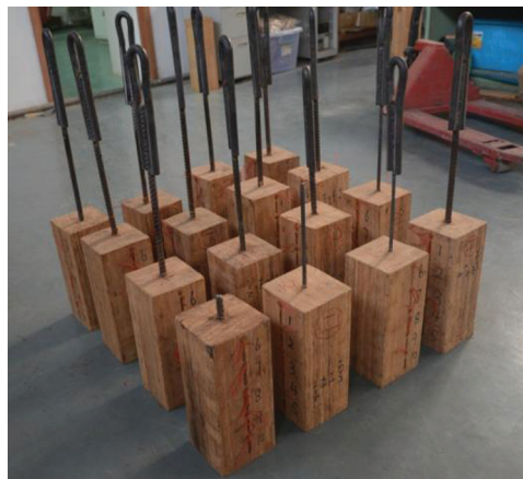
Figure 3: Anti pulling specimens after failure
