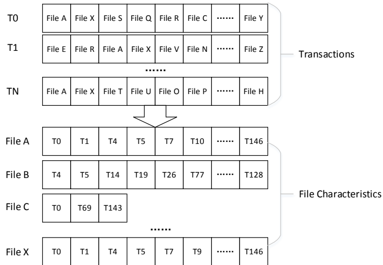
Figure 9: Inverted index for files with cache transaction
