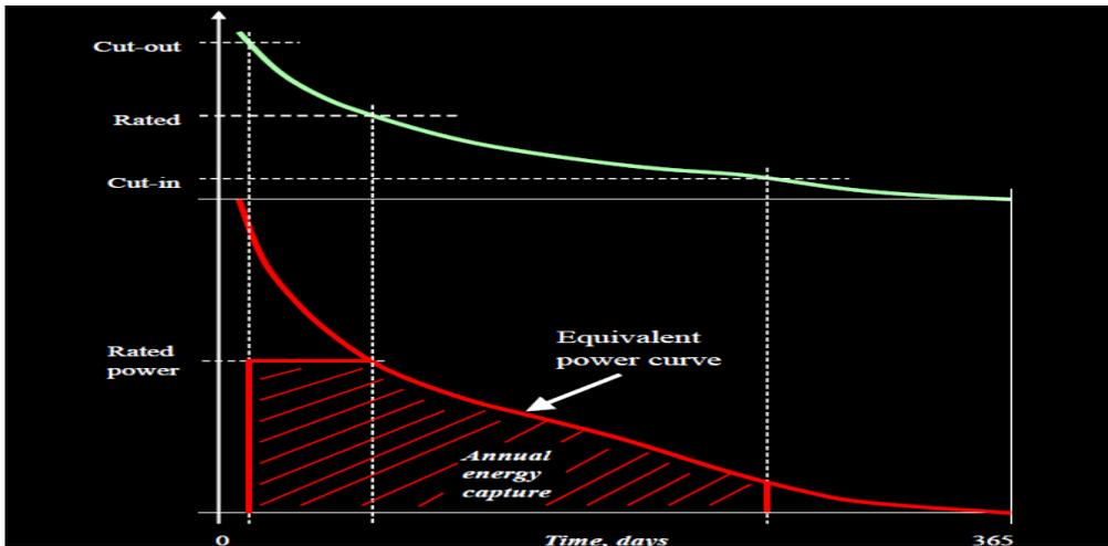
**Figure 4:** Power and speed curves of the turbine on daily basis
