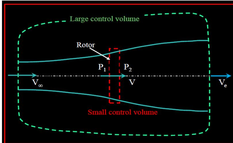
**Figure 2:** Control volume at the rotor, for derivation of the power equation by applying Bernoulli equation
