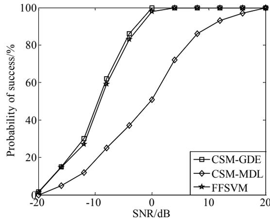
**Figure 4:** Accuracy vs. SNR for uncorrelated signals in colored noise
