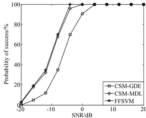
**Figure 6:** Accuracy vs. SNR for coherent signals in GWN
