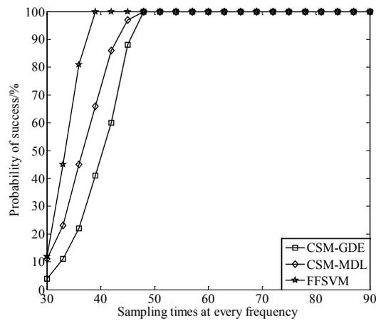
**Figure 7:** Accuracy vs. number of samples for coherent signals in GWN
