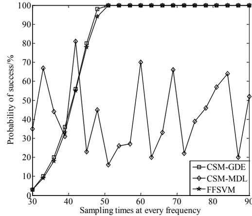
**Figure 5:** Accuracy vs. number of samples for uncorrelated signals in colored noise
