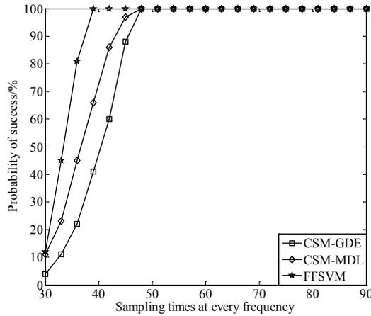
**Figure 3:** Accuracy vs. number of samples for uncorrelated signals in GWN
