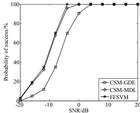
**Figure 2:** Accuracy vs. SNR for uncorrelated signals in GWN
