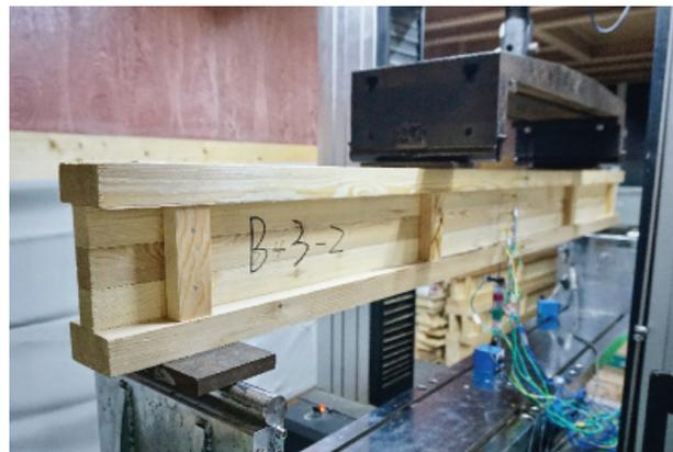
**Figure 2:** Four-point bending test-site of glulam beam (mm)
