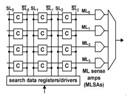
Figure 1: Simple schematic of a CAM
