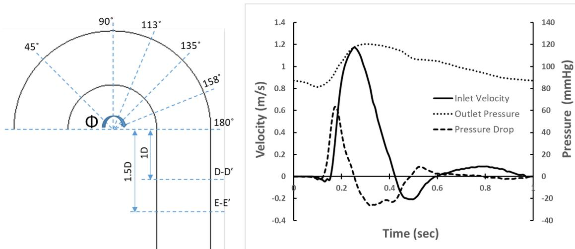
**Figure 1:** Schematic sketch of the curved tube and the prescribed inlet velocity and outlet pressure
