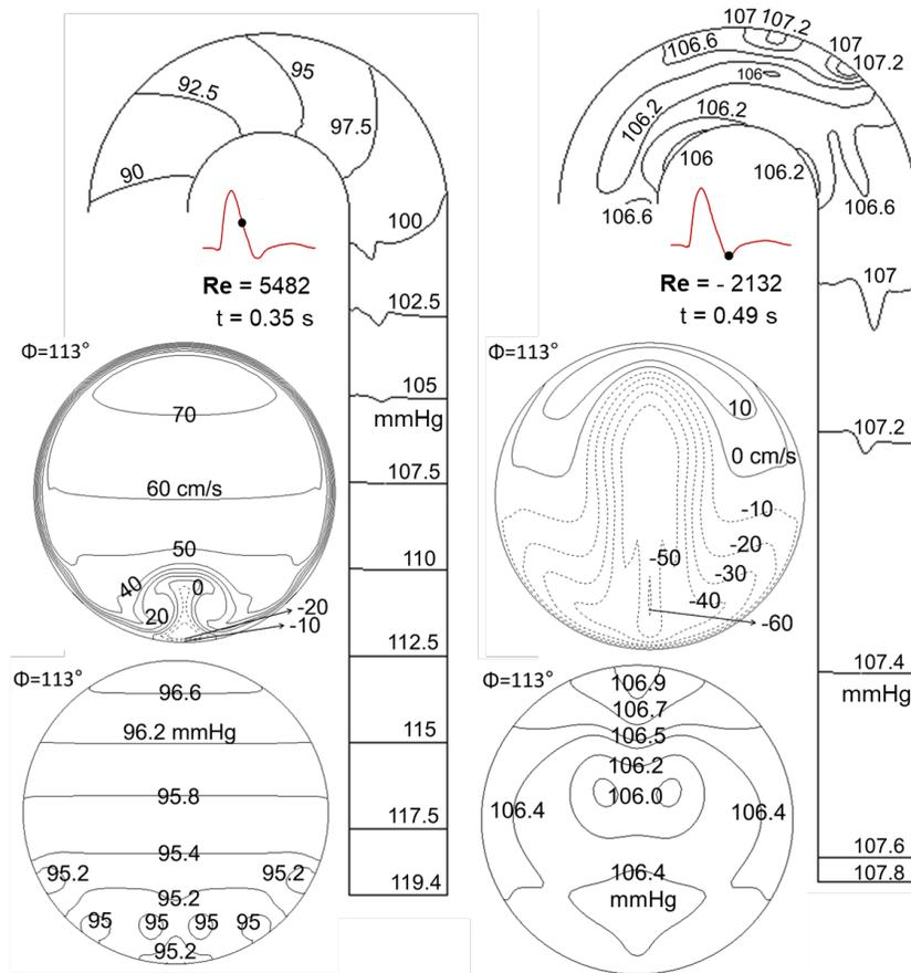
**Figure 4:** Longitudinal velocity ( $w$ ) and pressure contours at section  $\phi = 113^\circ$  on the symmetric plane for  $Re = 5482$  and  $-2132$
