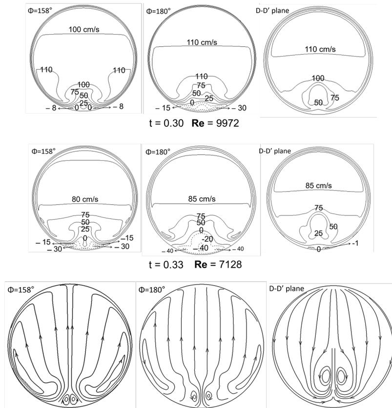
**Figure 3:** The longitudinal velocity contours and secondary flow patterns
