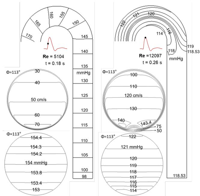
**Figure 2:** Longitudinal velocity ( $w$ ) and pressure contours at section  $\phi = 113^\circ$  on the symmetric plane for  $Re = 5104$  and  $12097$
