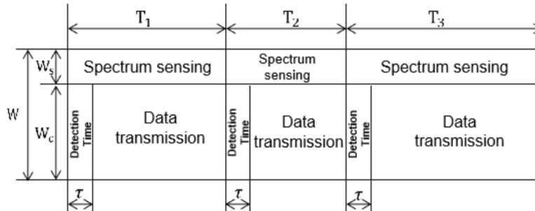
**Figure 2:** Sketch Map of spectrum segmentation technology
