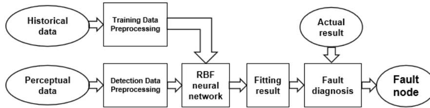
**Figure 5:** Fault detection flow chart based on RBF neural network
