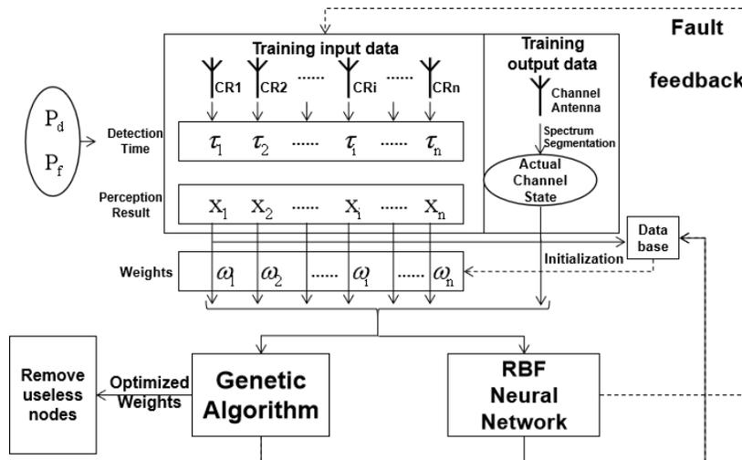
**Figure 1:** Centralized spectrum sensing model flowchart based on self-checking machine learning
