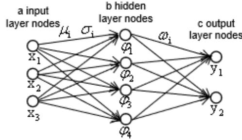
**Figure 4:** RBF neural network structure diagram
