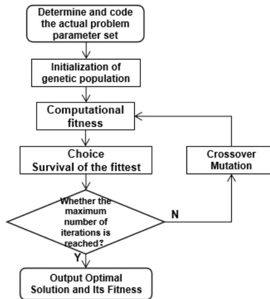
**Figure 3:** Genetic algorithm structure diagram
